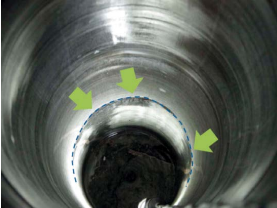
Figure 2-28. The location of inflows in KO0017G01, along a fracture identified at 2.9 m. See also the pegmatite vein that may conduct water. This figure is reproduced from the task description (Vidstrand et al. 2017).
