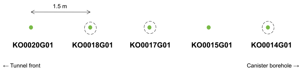
Figure 2-5. Illustration of probe borehole spacing and naming. This figure is reproduced from the task description (Vidstrand et al. 2017).
