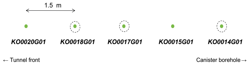
Figure 4-4. Illustration of probing borehole spacing and naming.
