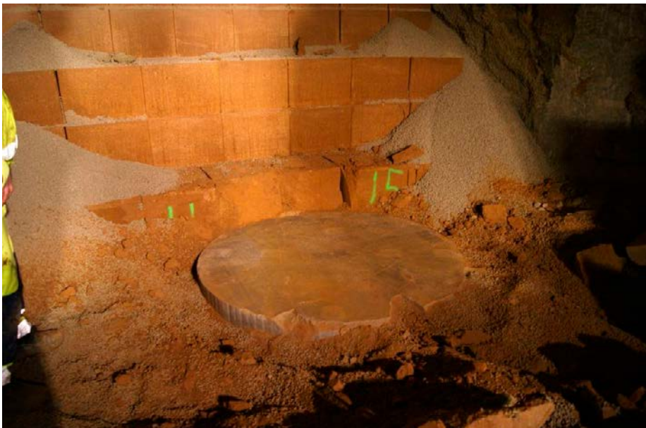
Figure 4-23. The buffer block is uncovered.
