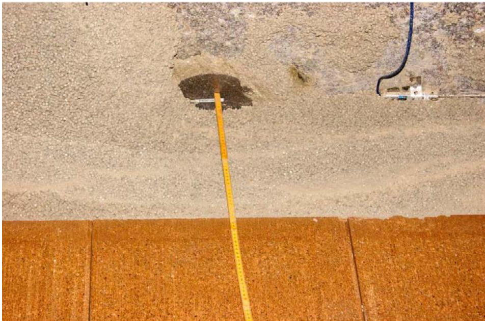
Figure 4-28. The distance between block stack and the pressure sensor (1) was determined to be 383 mm after test. .
