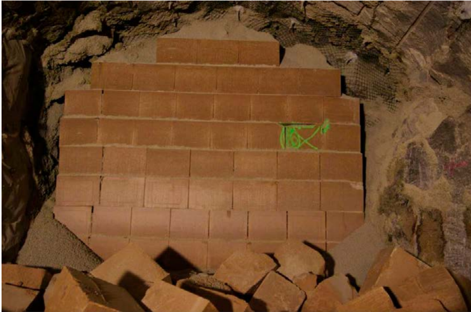
Figure 4-22. The block stacks inside the deposition hole beyond vertical section 1 are almost unaffected by the buffer heaving.
