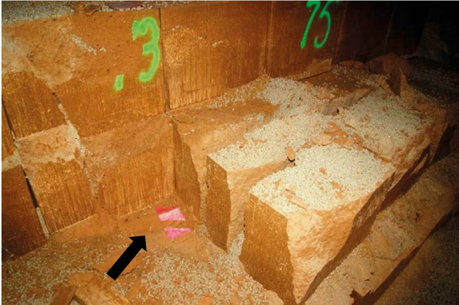
Figure 4-10. The pressure indicator on the photo was positioned on top of layer 3. The block below has been sheared and the shear surface can be seen very evidently (black arrow). Parts of the block have been vertically sheared approx. 50–60 mm relative the rest of the block.
