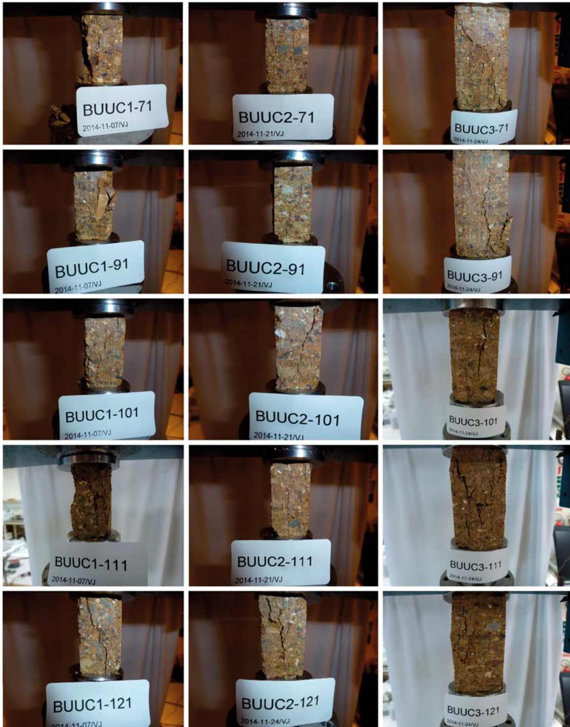
Figure A4-1. Post-failure photos from series 1 (BUUC1 – column to the left), series 2 (BUUC2 – the middle column) and series 3 (BUUC3 – column to the right). Each row show photos of samples from the same block, i.e. 7–12, except 8.
