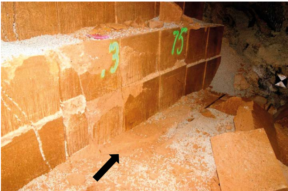
Figure 4-11. Some additional blocks of the ones shown in Figure 4-10 have been removed and the shear surfaces can be seen clearly (black arrow at the top on block layer 3).
