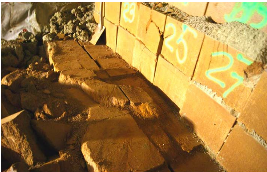
Figure 4-19. Shear surfaces on vertical block layer 3. See also Figure 4-11.
