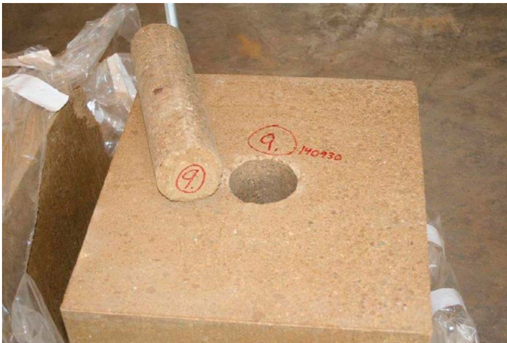
Figure 6-2. A core with diameter 100 mm has been drilled out from the block centre.
