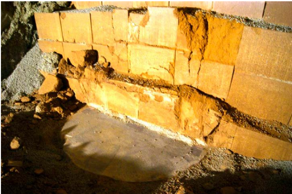
Figure 4-26. Photo showing the middle part of the buffer block together with the compressed pellet and backfill blocks (same as Figure 4-20).
