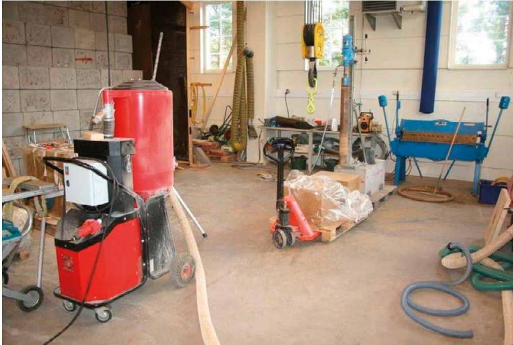
Figure 6-1. Arrangement for the block sampling. The core drill is seen in the back of the picture and the vacuum cleaner, used for removing dust, in the front.
