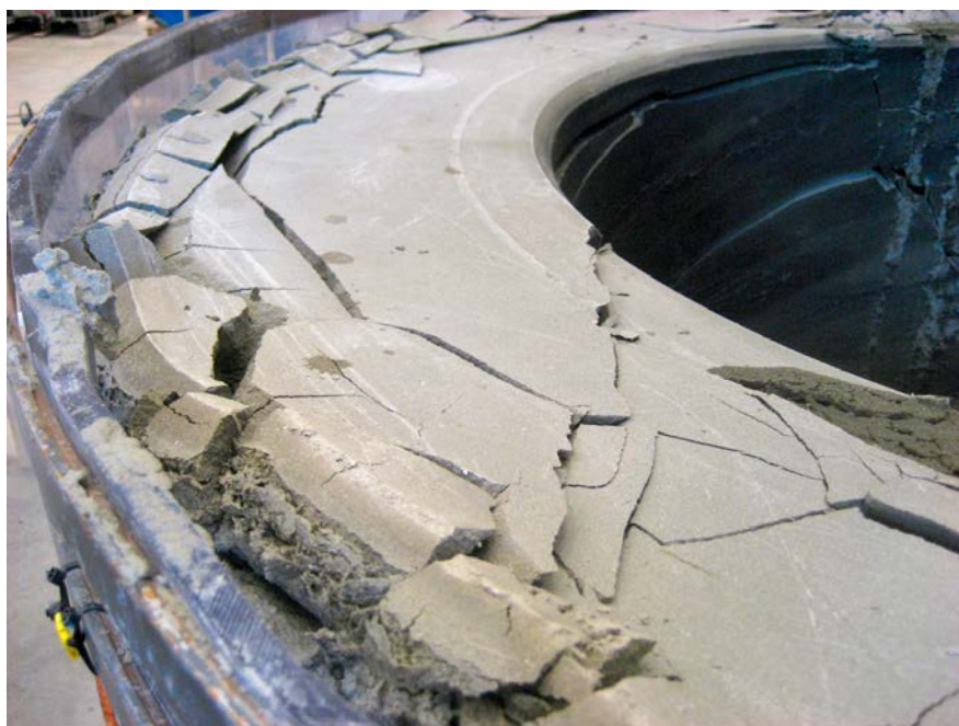
Figure 2-9. Deformation damage in a bentonite block without vertical load in a situation with artificial water supply (Åberg 2009).
