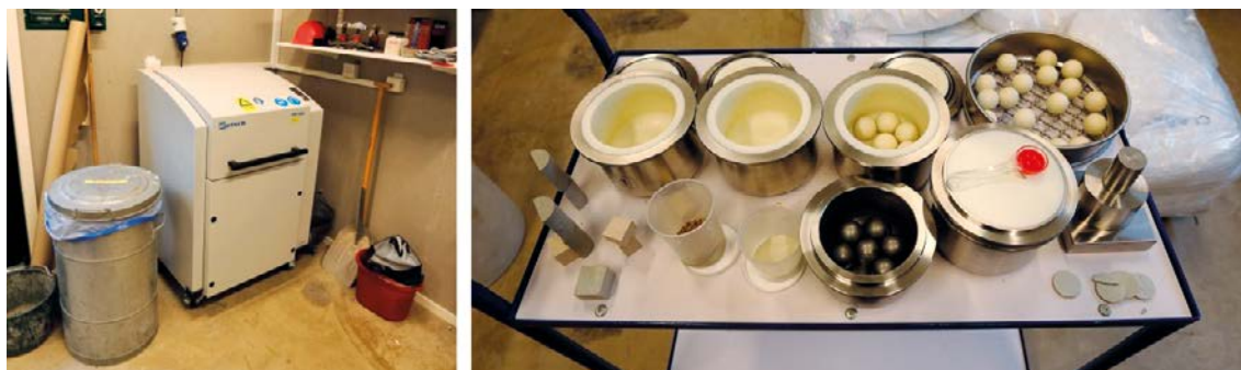
Figure 7-1. Ball mill equipment. Right: Different inserts for ball mill of zirconiumoxide and stainless steel. To the right of the table the compaction mold for the XRF samples can be seen.
