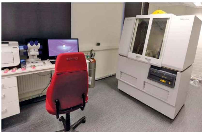
Figure 9-1. X-ray diffraction equipment at Åspö clay science laboratory. The microscope is used for sample preparation.
