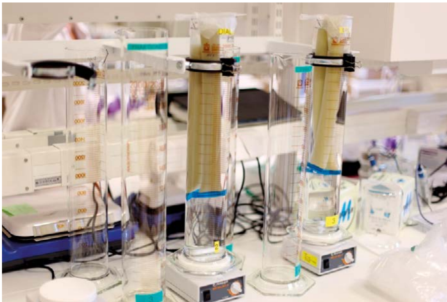
Figure 7-2. Purification of clay fraction using dialysis to remove salts. This is a very slow process that normally takes some weeks.
