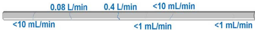
Figure 4-6. Case KBS-3H Median inflow drift of length 300 m. Inflows and inflow positions are shown.
