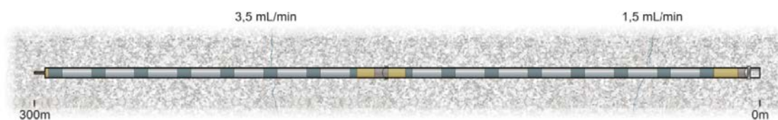
Figure 4-20. Schematic drawing of the KBS-3H drift design in the dry case.
