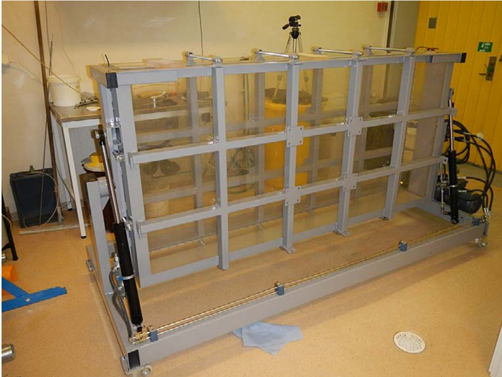
Figure 2-3. Photo showing the further developed large slot test equipment (B+tech Oy).
