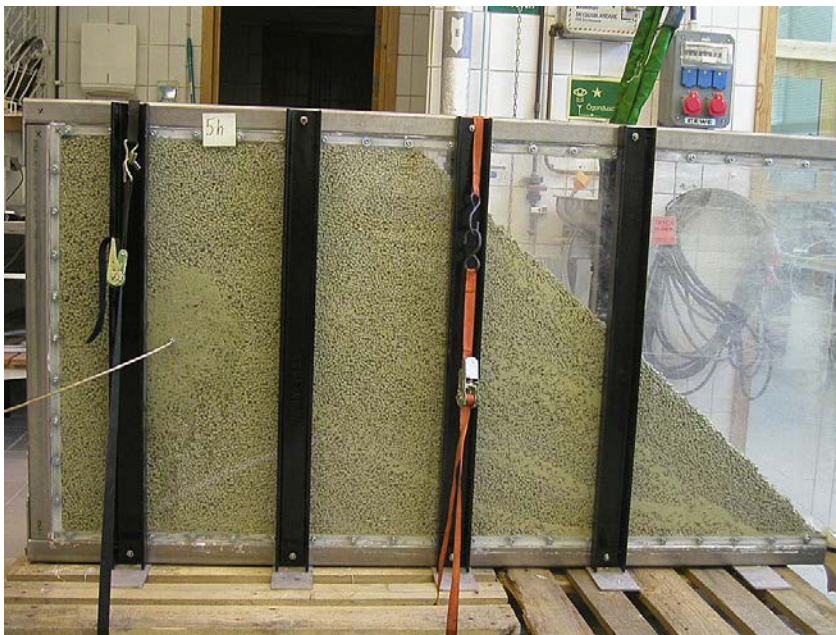
Figure 2-2. Picture showing the test equipment designed at Clay Technology AB. The slot is open on the short side to the right. A constant inflow can be applied at the mid height, see tube connection in photo.
