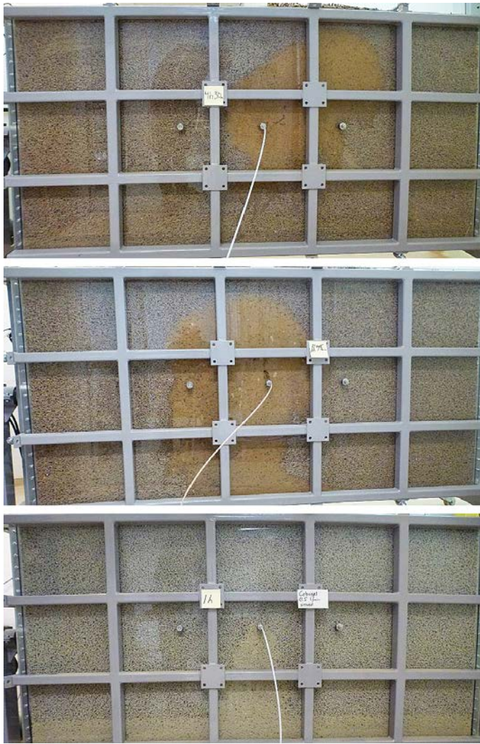
Figure 2-9. Upper: Photo showing an example of “Symmetric/Upwards” wetting. Middle: Photo showing an example of “Symmetric” wetting. Lower: Photo showing an example of “Downward” wetting.
