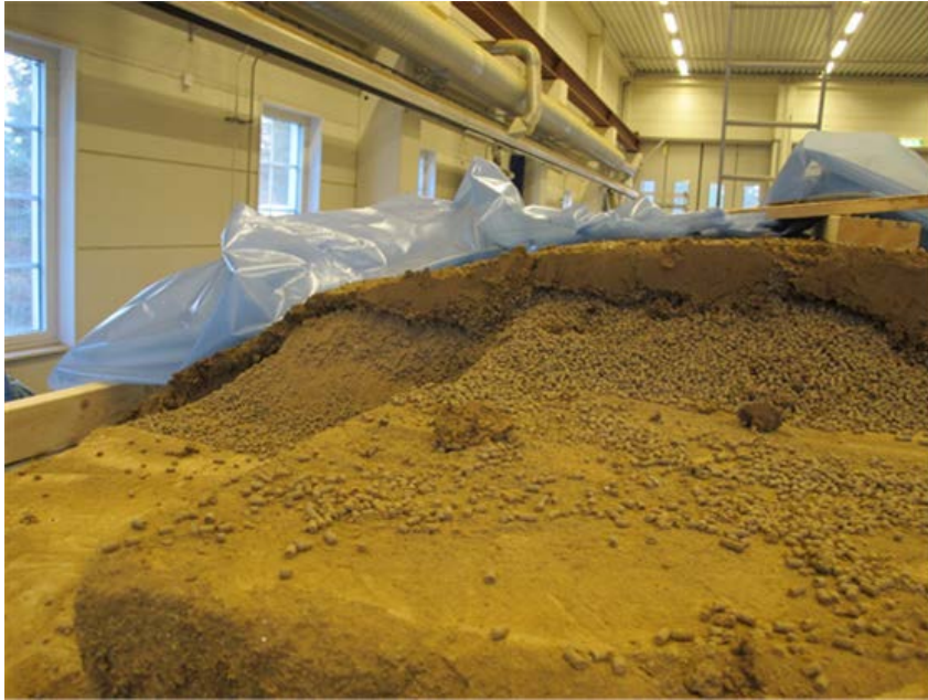
Figure 2-13. Photo showing a cross section (close to the installed geotextile) of the pellet filling at the top of the tunnel in Test 5. It is obvious that the inflowing water has followed the geotextile up over the crown and down on the other side of the tunnel (inflow side to the left in the photo). However, as shown in the photo, there is a remaining dry layer of pellets close to the block stack.
