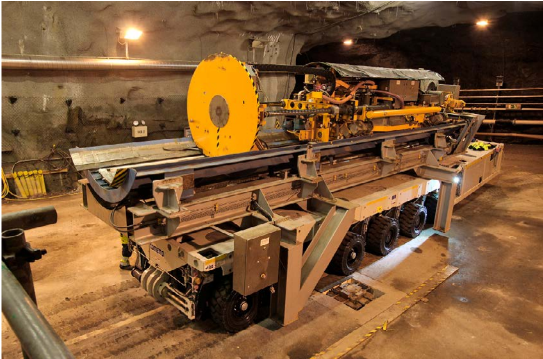
Figure 7-6. Starting tube with the deposition machine being moved into position by MODE.
