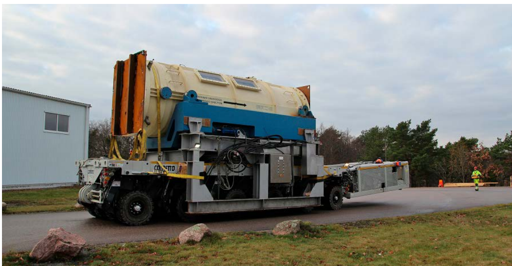
Figure 7-5. Transport tube secured to MODE transport vehicle being ready for transport down to the deposition drift at -220 m.
