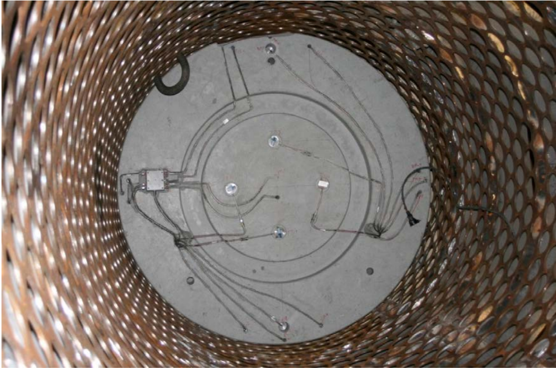
Figure 8-6. The bottom block inside the Supercontainer with all cabling through diagonal holes and into the cable block. For the Supercontainer the wireless transmitter that can be seen to the left had an antenna extending outside of the shell to avoid any Faraday's cage effects.
