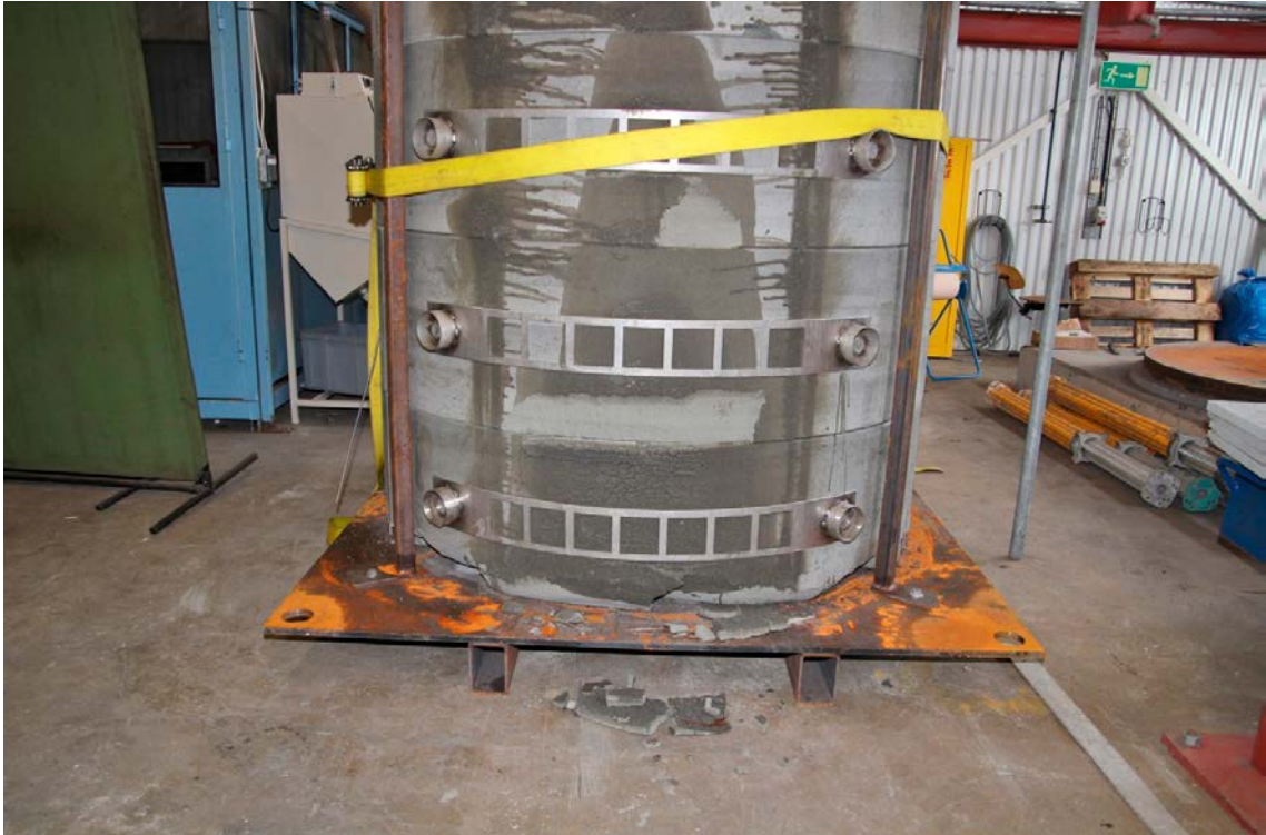
Figure 7-9. Test distance block back in the assembly facility, the effects of splashing is evident.
