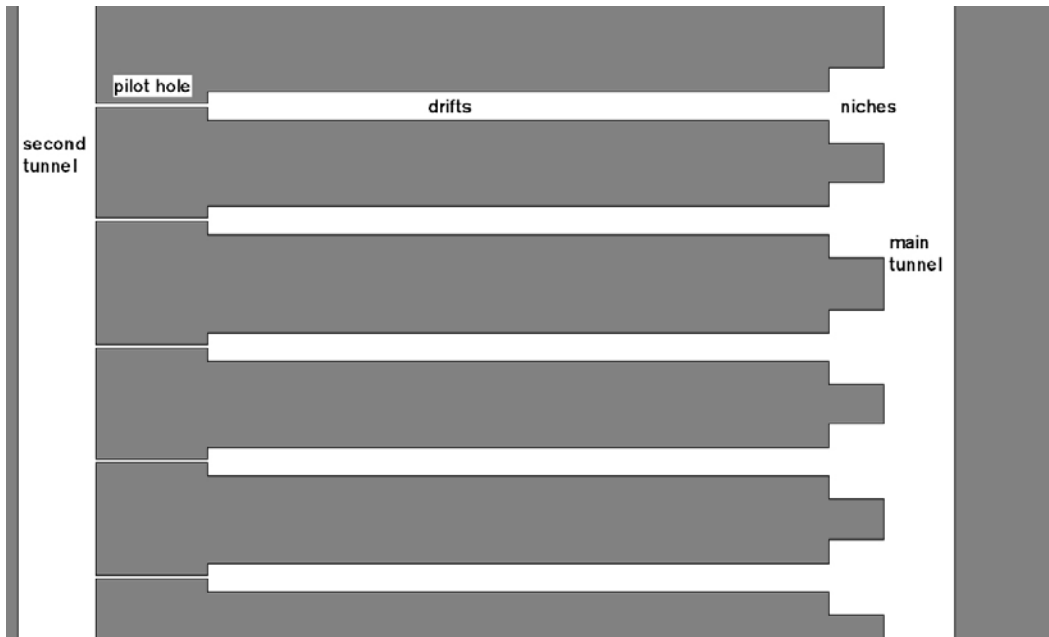
Figure 11-1. Schematic illustration of a double tunnel system, drifts are reamed between two tunnels, rock 'cover' is left in the end and only the pilot hole has to be plugged at that side.
