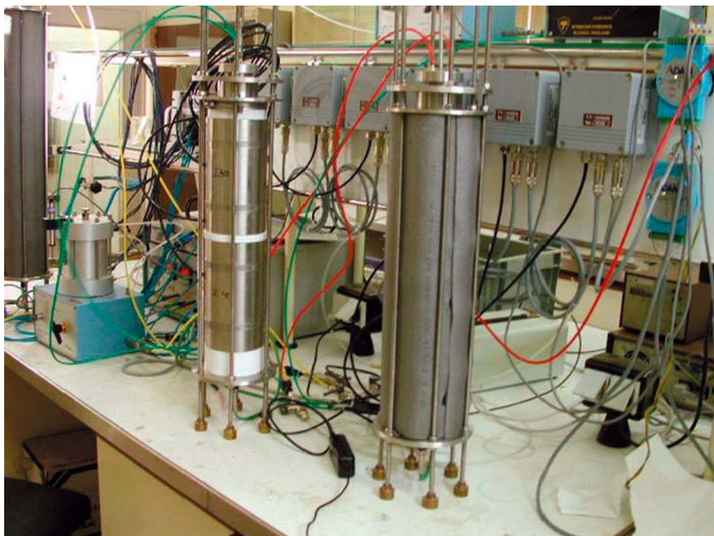
Figure 3-1. Large infiltration cells: isothermal test (left) and thermal gradient test (right).
