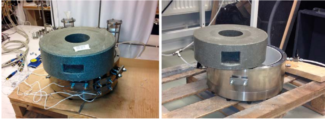
Figure 6-4. The cylindrical bentonite block used in the tests SH1 (to the left) and SH2 (to the right) with cut cavities. In the diametrical position of each block a second cavity was cut. The dimensions of the cavities in SH1 and SH2 were (height \times length \times depth) (35 \times 70 \times 50) \text{ mm}^3 and (50 \times 70 \times 50) \text{ mm}^3 , respectively.
