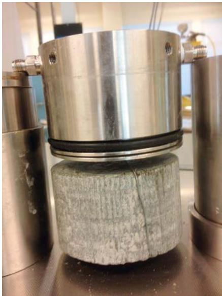
Figure 5-58. Photo of the specimen, suspended in the upper piston, before mounting into the test device.
