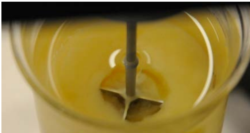
Figure 5-2. Ku-mmt, 20 g/l in 20 mM NaCl(aq) after a yield stress measurement.
