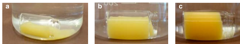
Figure 4-1. Three gels after rapid heating to 75 °C. (a) Ku-Na gel (10 g/l) in 5 mM NaCl solution. The gel underwent almost complete melting transition during heating to 75 °C and solidified as the temperature was lowered. (b) Ku-Na gel (10 g/l) in 6 mM NaCl-solution. The gel experienced large deformation (partial melting) during heating to 75 °C. (c) Ku-Na gel (20 g/l) in 200 mM NaCl-solution. The gel showed no sign of change.
