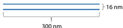
Figure 1-4. Side view of two montmorillonite layers at a separation where the van der Waals attraction is of the order of k_B T .
