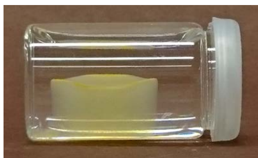
Figure 1-5. Snapshot of Ku-Na gel taken ca seven years after formation in a mixed NaCl/NaOH solution of ionic strength 15 mM and pH \sim 11 . Initially the vial was standing upright and filled with a montmorillonite sol of 2 g clay/l that was settling and slowly gelling and consolidating. After the gel was formed, the vial was placed horizontally and the gel eventually unfastened from the glass and flipped forward. Most of the clay particles actually settled before gelation took place. Based on turbidity we estimate the clay concentration in the gel to be less than 2 g/l, equivalent to a volume fraction of 0.07 %. Note that the gel is fully surrounded by electrolyte.
