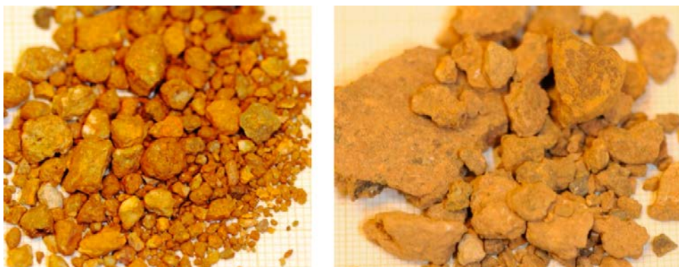
Figure 5-3. Photos showing the difference in granule shape between Asha 2010 and Asha 2012. Left: Close up of the Asha 2010 material Right: Close up of the Asha 2012 material.
