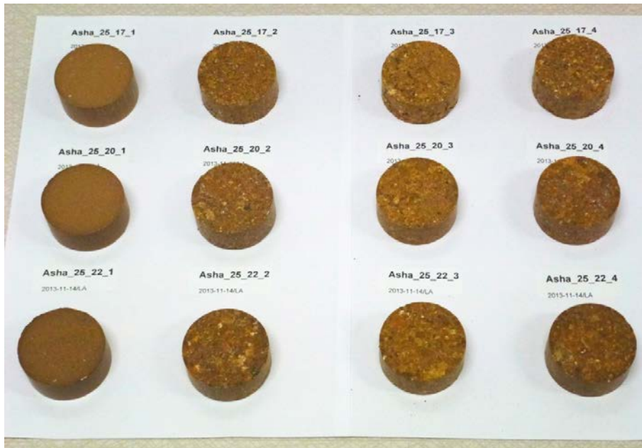
Figure 6-2. Photo showing Asha specimens compacted with 25 MPa.
