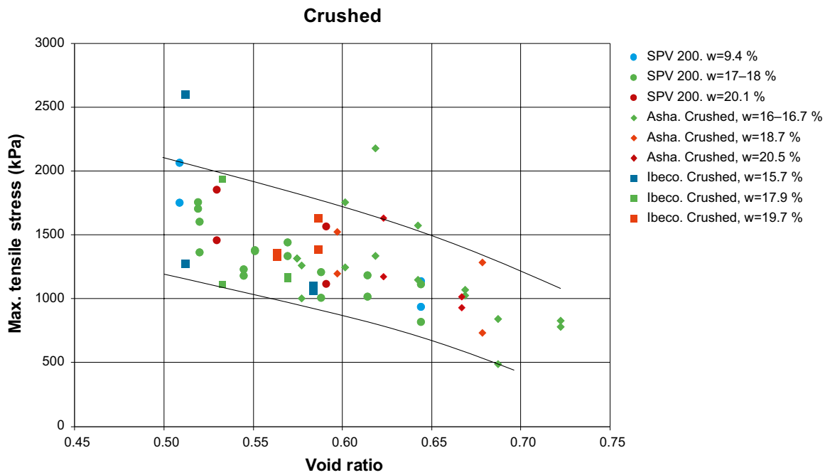
Figure 6-10. The determined maximum tensile for the fine and crushed materials plotted versus void ratio.
