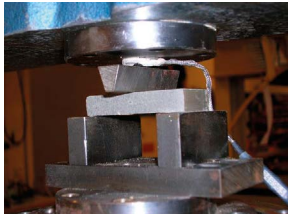
Figure 6-1. Test arrangement for determination of the tensile strength.
