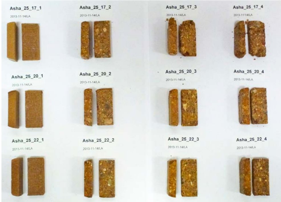
Figure 6-4. Photo showing beams of Asha specimens compacted with 25 MPa.
