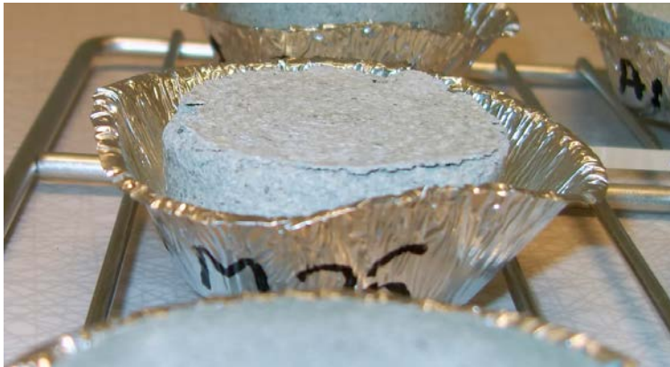
Figure 7-10. Photo of A12 M 75 where the top surface started to peel off.
