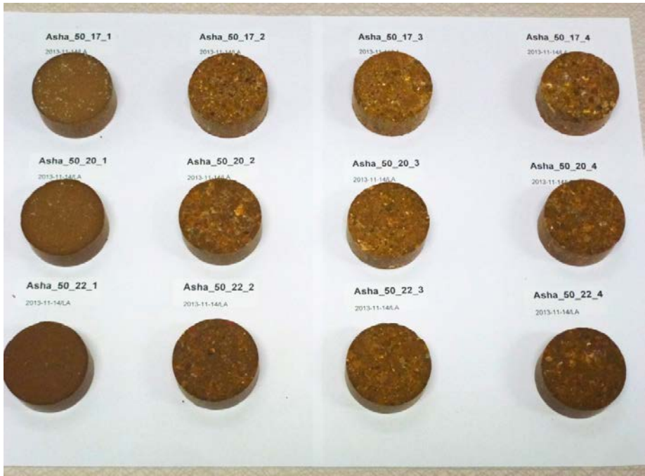
Figure 6-3. Photo showing Asha specimens compacted with 50 MPa.
