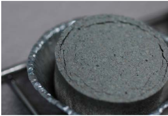
Figure 7-14. Circular cracks in A12 S 95 after 2 hours.
