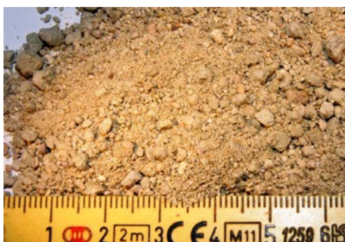
Figure 5-4. Close up of the granules in the as-delivered material from the Ibeco 2011 batch.
