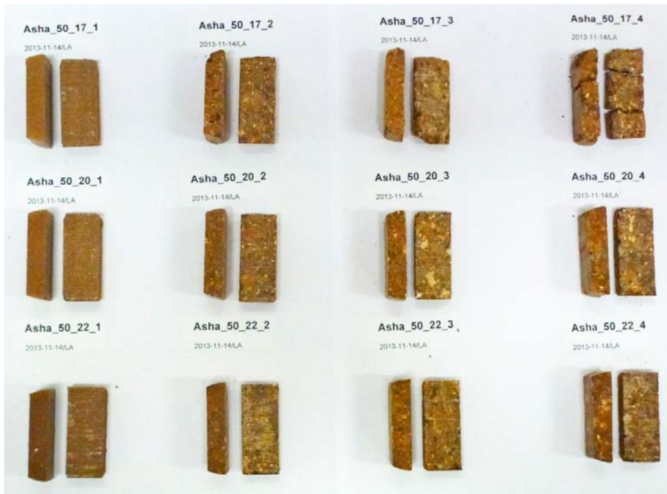
Figure 6-5. Photo showing beams of Asha specimens compacted with 50 MPa.
