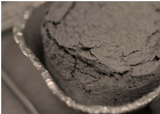
Figure 7-15. Cracks in A12 M 95 after 168 hours.
