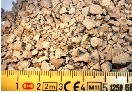
Figure 5-5. Close up of the granules of crushed MX-80 pellets.
