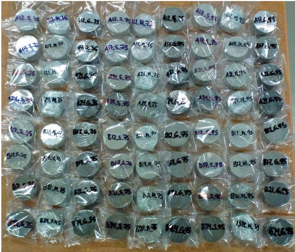
Figure 7-2. All the prepared specimens. The specimens are packed in double plastic layers after manufacturing.
