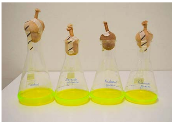
Figure 3-1. Growth cultures and control with 20 \text{ mg L}^{-1} uranine. From left: the control, Shewanella putrefaciens , Pseudomonas stutzeri , and Pseudomonas fluorescens .
