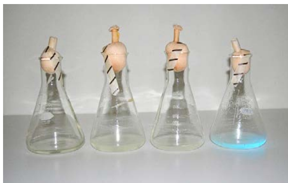
Figure 3-3. Growth cultures and control with 40 \text{ } \mu\text{g L}^{-1} uranine irradiated with UV-light, demonstrating pyoverdine production. From left: Control, Shewanella putrefaciens , Pseudomonas stutzeri , and Pseudomonas fluorescens .
