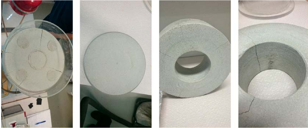
Figure 2-21. Excavation of test 6. Left: The top of the massive top block. Second to left: bottom side of the top block. Second to right: bottom side of the top ring. Right: top side of the bottom ring.
