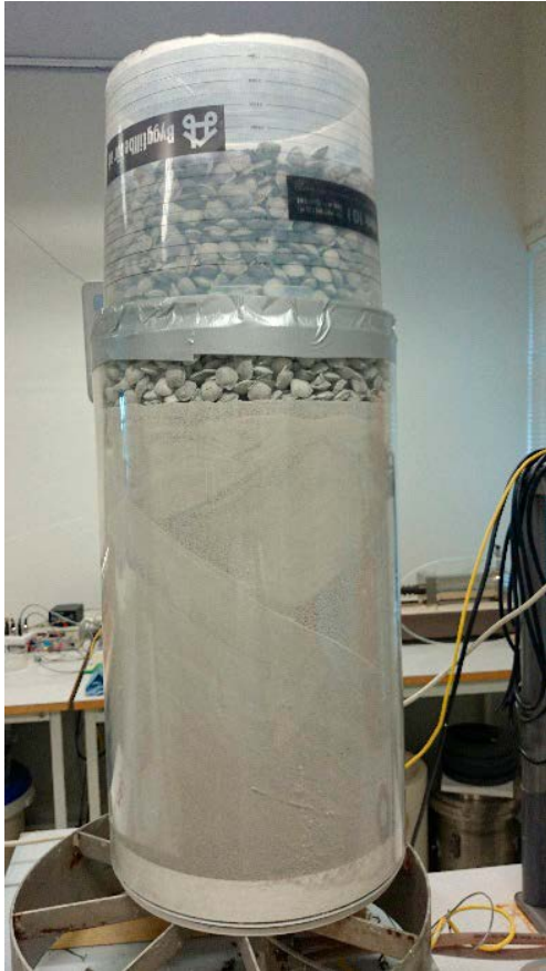
Figure 2-25. Test 7 with a 20 cm thick pellets filling replacing the rubber mat as top seal.
