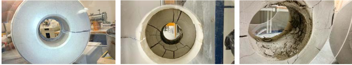
Figure 2-11. Test 4 at termination. Left: the top side of the top ring. Middle: Top side of bottom ring. Right: Bottom side of bottom ring.
