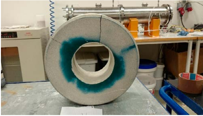
Figure 2-16. The mid ring seen from the top side. The blue coloring is due to a plastic mat which was placed in between this and the top ring in order for the blocks to line up with the copper tube.
