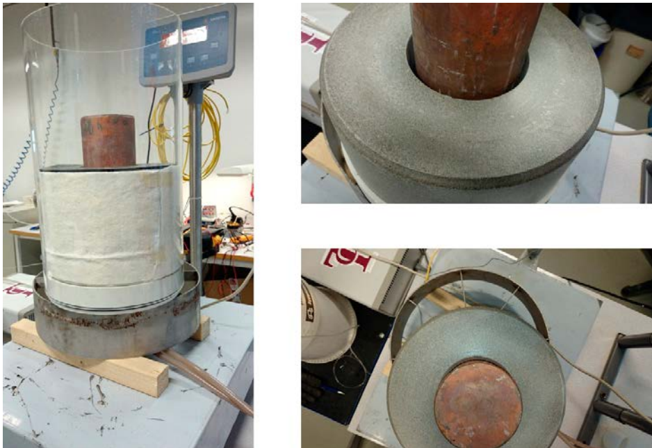
Figure 2-9. Test 4 at the start of the test. The top ring had an inner radius small enough as to basically seal off the inner slot (bottom right).
