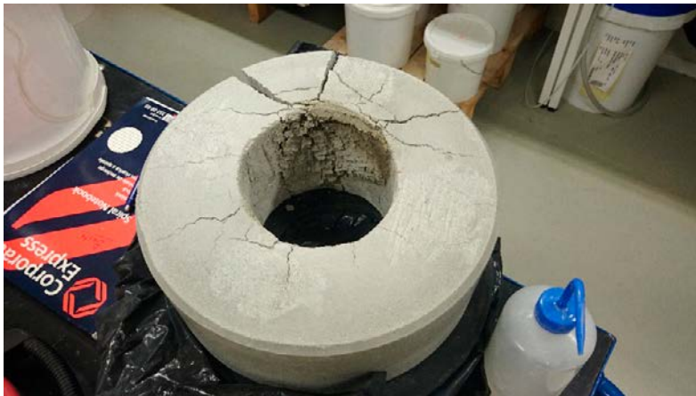
Figure 2-5. Bottom side of the bentonite ring in test 2 after termination. Vapor has been taken up unevenly, by local condensing.
