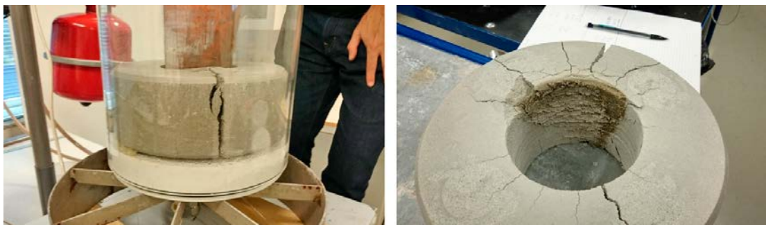
Figure 2-8. Left: Test 3 at termination. Right: Bottom side of the bentonite ring showing a condensation “nucleus”.
