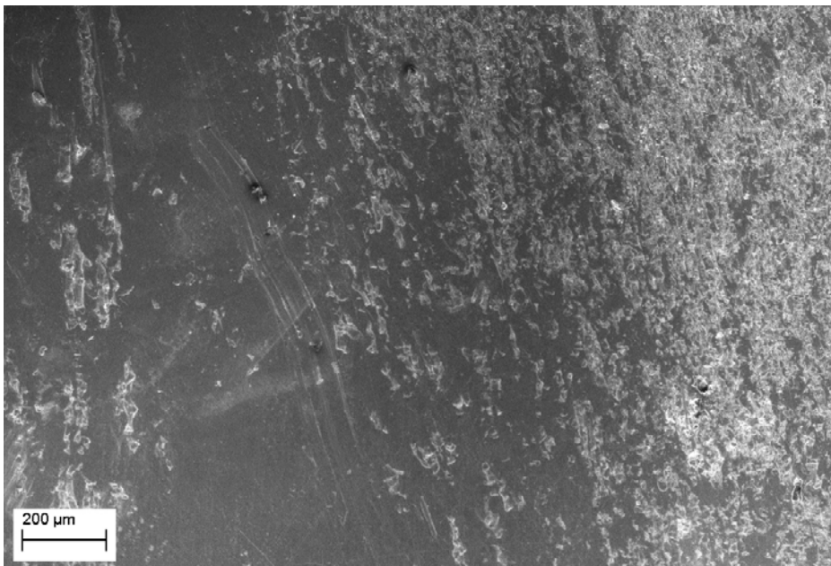
Figure 3-29. Copper surface after scratching with diamond (as in sample M2-diam). The right side with a heavily disturbed surface might show the effect of impressions by diamond particles, not detectable themselves in SEM.
