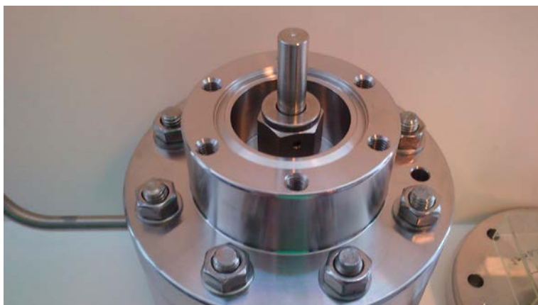
Figure 2-3. The new lid, here with blind VCR 1/4" connection together with the outer CF-38 seal.
