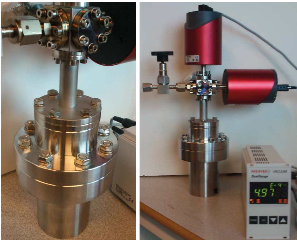
Figure 2-1. A new setup for pressure measurements (Main 3) equipped with a new lid including the Pd membrane (cf. Figure 2-3). The outer diameter of the lower chamber has been reduced.
