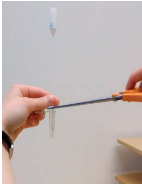
Figure 2-3. Sampling with swab on fracture surface to detect ATP, indicating the number of living cells. 1. Water-conductive fracture surface detected in a drillcore. 2. ATP extracting reagent is added to the surface. 3. Released intracellular ATP is collected with swab. 4. The top of the swab is put into an Eppendorf tube and stored in freeze until analysis.
