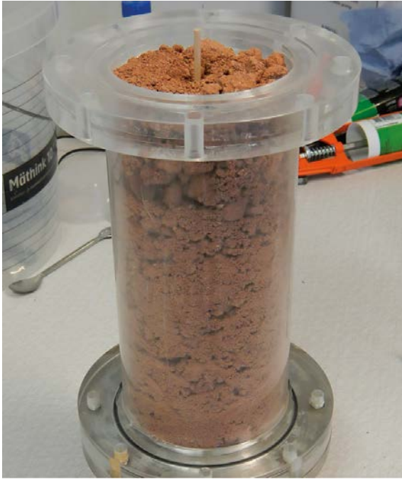
Figure 2-5. Sample preparation with a 4 mm stick to artificially create a flow channel.
