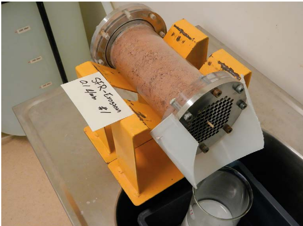
Figure 2-4. The fully rigged test equipment. A transparent tube with inner diameter 100 mm and length 250 mm was used in all tests.
