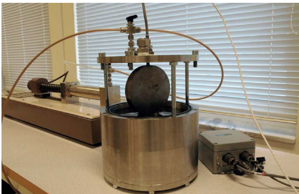
Figure 4-4. Test cell with a total pressure sensor before immersion into water (Nilsson 2014).
