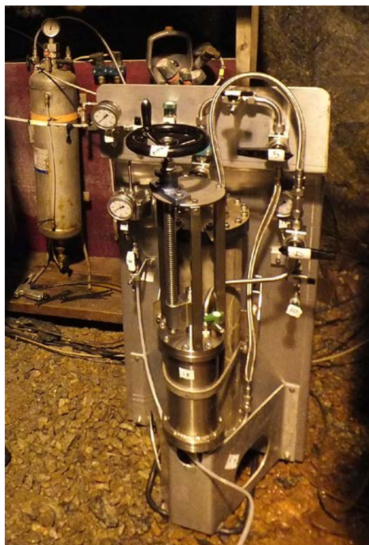
Figure 7-20. Sampling vessel for preservation of RNA from borehole water maintained under in situ conditions.
