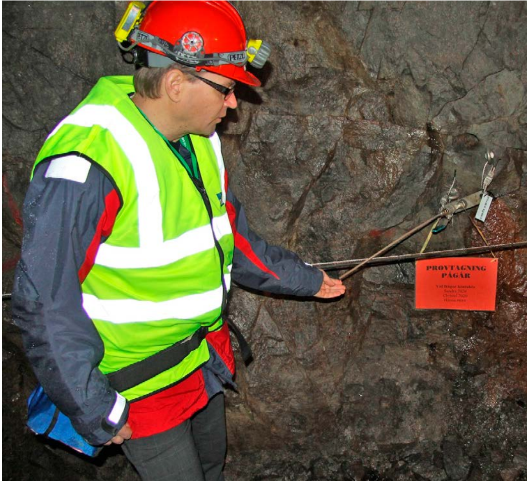
Figure 7-3. Sampling of fracture groundwater for characterization of dissolved concentrations of lanthanoids. Photo: Tobias Berger.
