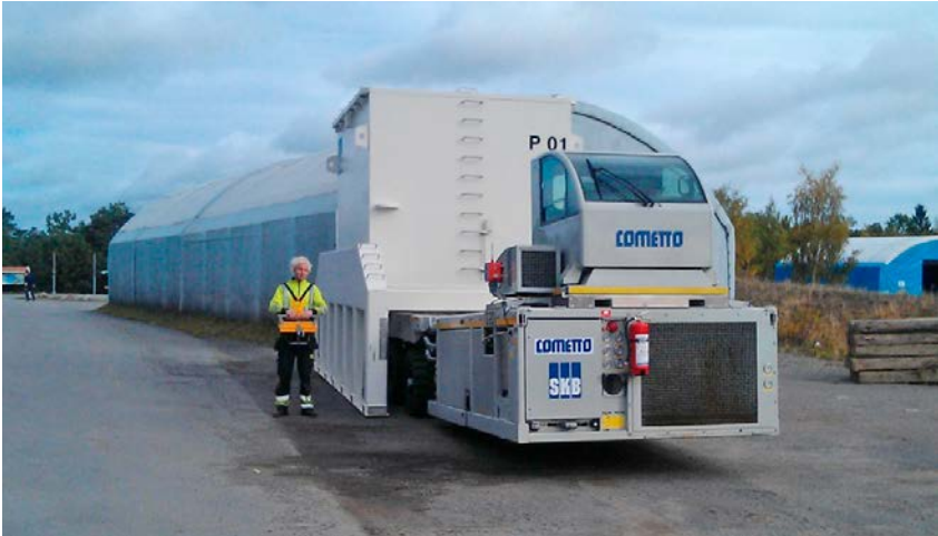
Figure 5-6. Ramp Vehicle carrying the modified ATB.
