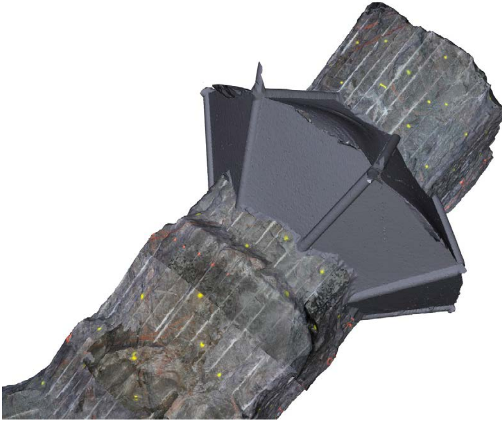
Figure 4-30. Illustrative model structured of data from laser scanning of TAS01 as well as of the excavated slot abutment (seen from above).
