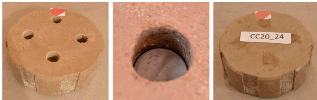
Figure 4-15. Final preparation of a bentonite block. Left image shows how the block has been given its final shape with slits made to fit with the titanium cage and holes drilled for the small sample cylinders. In the centre image a cement cylinder has been placed in the small hole and the right image finally shows how the holes have all been filled with bentonite powder of the same type as the bentonite block itself.
