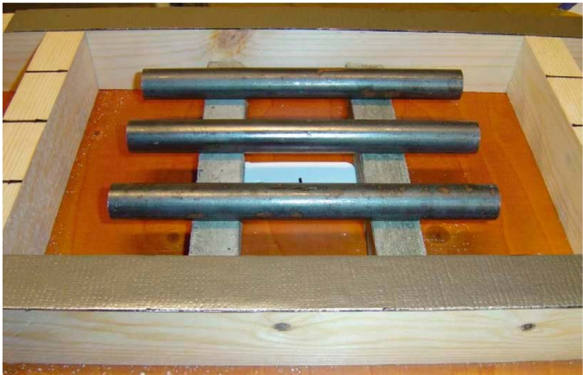
Figure 4-20. Mould and steel bars on support before casting.
