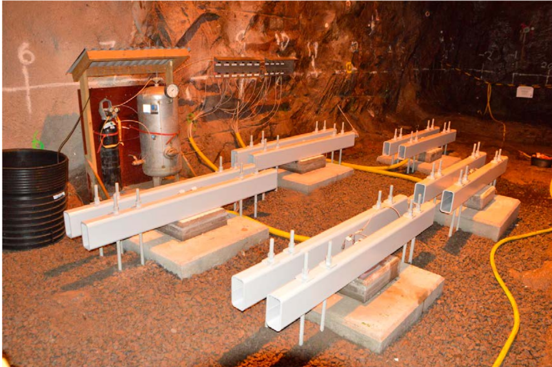
Figure 4-18. Installation completed and system for artificial saturation of the experiments connected.
