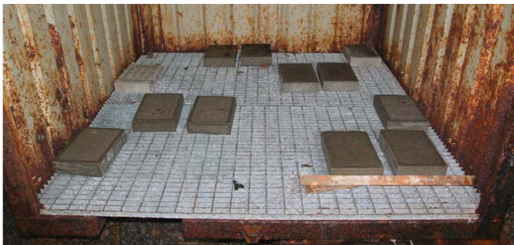
Figure 4-21. Container in Äspö HRL with corrosion tests samples.
