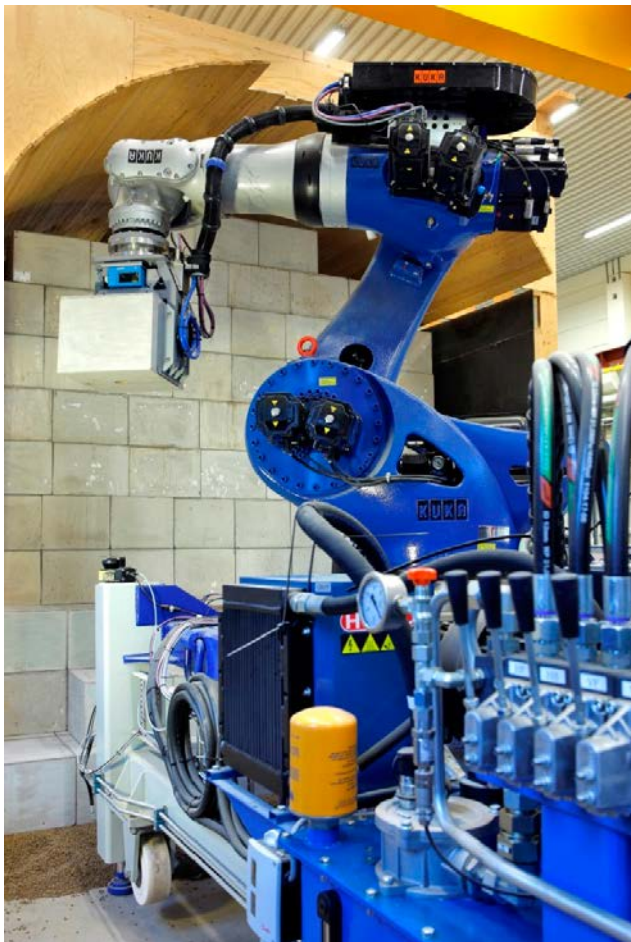
Figure 4-25. A photo of KUKA KR 1000 L750 Titan, the prototype robot for installation of backfill.
