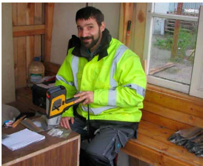
Figure 7-25. Dr Fabioc Kaczala using the XRF-instrument.
