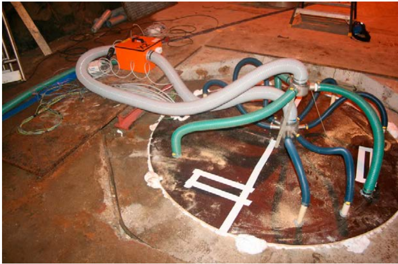
Figure 4-37. Lid on top of deposition hole. Inlet pipes are blue, out let pipes are green and dehumidifier is orange.
