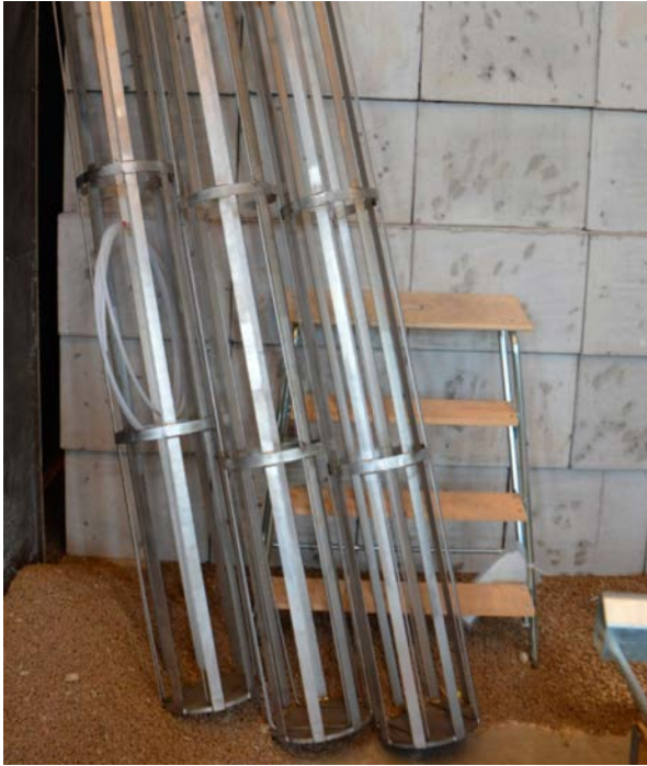
Figure 4-16. The lower part of three of the titanium cage used in the large scale bentonite experiments.
