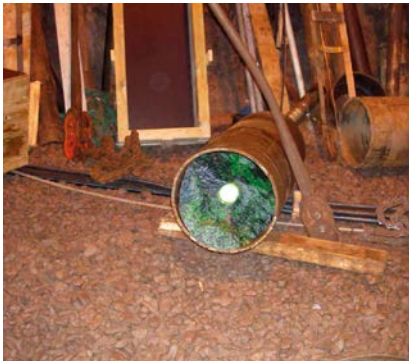
Figure 3-18. Core recovery barrel on ground level beside drill rig with core capturing ring still attached to the barrel, containing a core piece from KXTT3, showing the fracture at 13.9 m (looking up hole), with chlorite (black) and some epoxy (green) filling.
