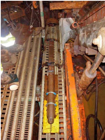
Figure 3-12. A sledge constructed on site for core breakage, sliding the tool for core breakage into the borehole above the core.
