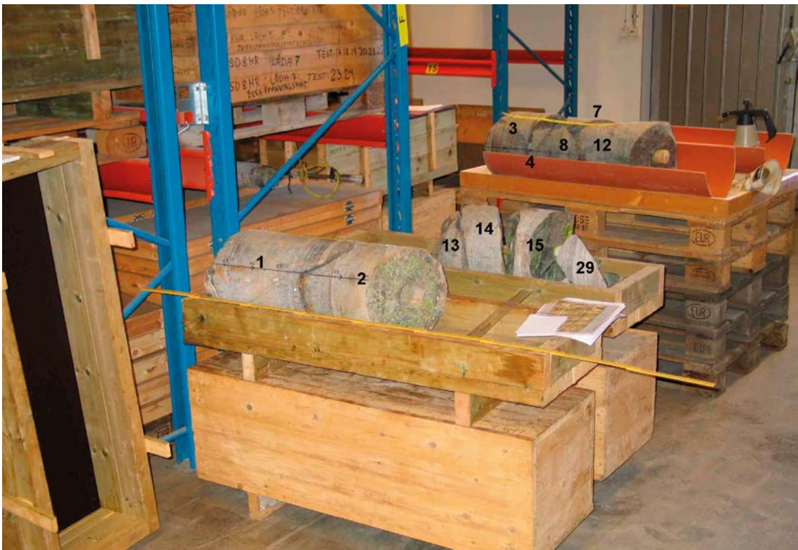
Figure 3-23. Mapping of core pieces from target area of KXTT3 in progress in core boxes in the core shed at the Äspö HRL. Numbers of identified core pieces can be seen and black orientation line on core pieces #1 and #2 which indicates vertical down of core.
