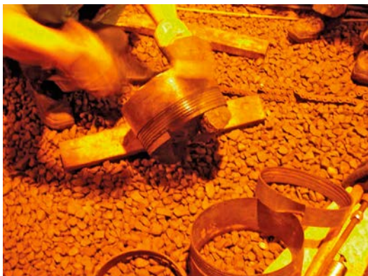
Figure 3-17. Drillers extracting core piece from the capturing ring at the end of the core recovery barrel.
