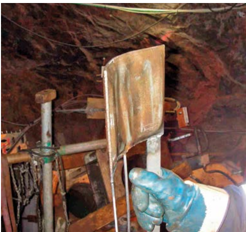
Figure 3-11. Tool for inducing core breakage, double steel plates (after being expanded using hydraulics, up to 80 bars).
