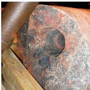
Figure A6-11. The overcoring of borehole KXTT4 at the TRUE-1 site. The deviation at approximately 10.2 m drilling length is approximately 44 mm of to the side.
