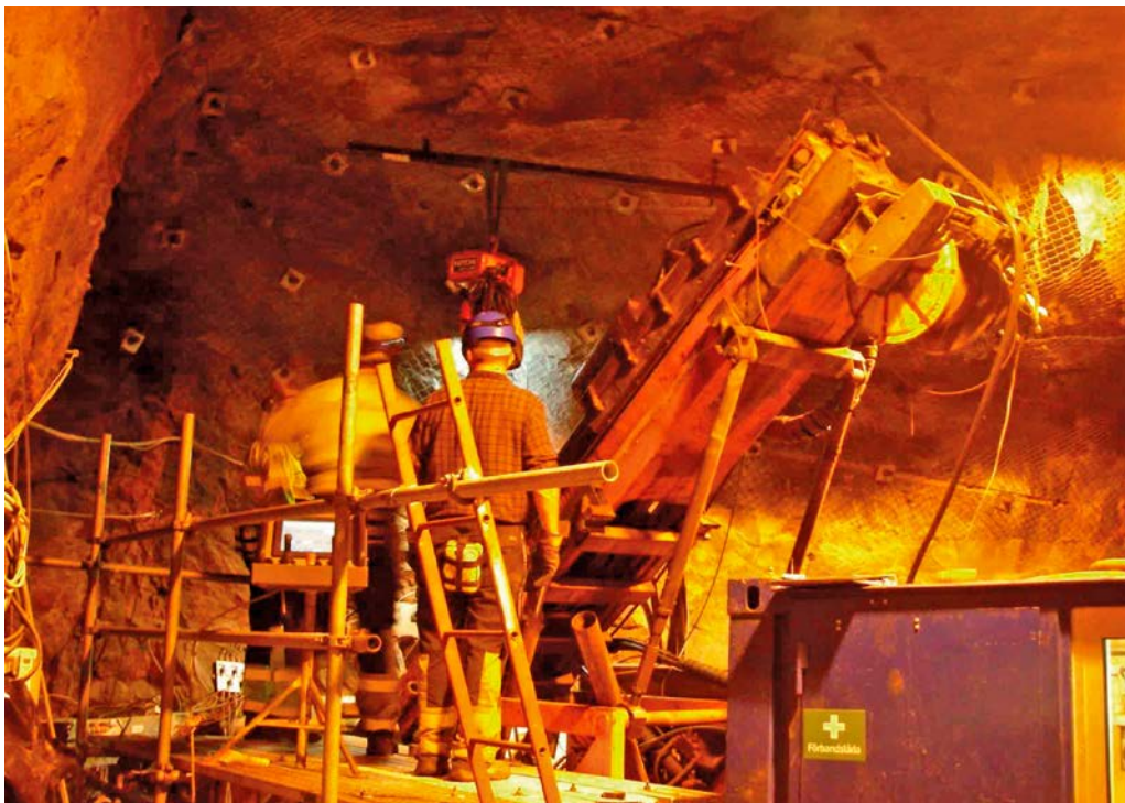
Figure 3-5. The Onram 2000 CCD computer controlled drill rig used for the overcore drilling of KXTT3 and KXTT4. The screen of the computer-aided control unit can be seen centre-left, behind the drillers.
