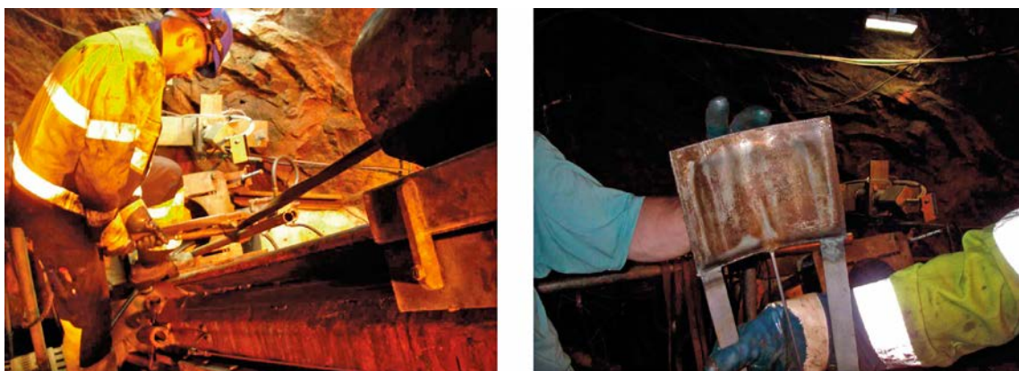
Figure A6-4. Drill site of TRUE-1, core breaking in KXTT3. (a) Disconnecting core breaking sledge (for breaking core from below) from drill string. (b) Core breaking device after being inflated to 80 bars.
