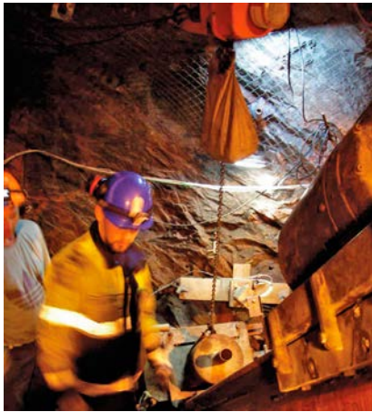
Figure 3-15. Core recovery barrel fastened to lifting device above drill rig for hoisting from the borehole to the drill rig platform.
