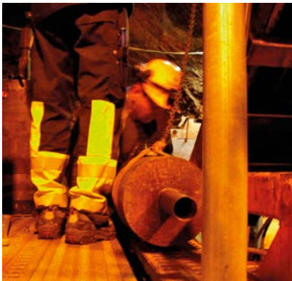
Figure 3-16. Core recovery tool on drill rig platform, drillers preparing for lowering the core recovery barrel with core down to ground level beside drill rig.
