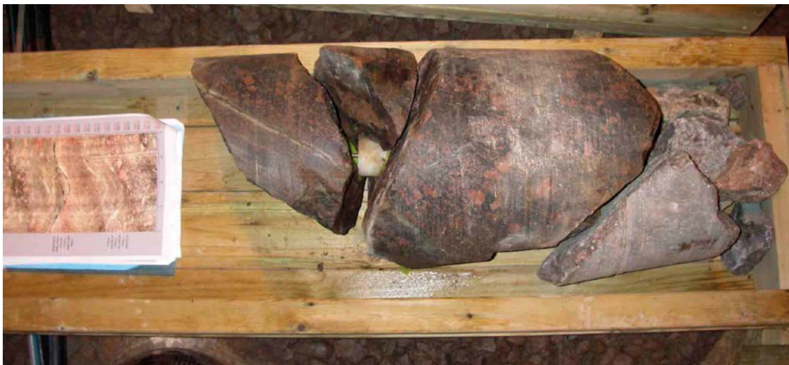
Figure 3-21. Core pieces from target section of KXTT3 in core box at drill site, paper print of BIPS image left of core in core box. Subsequent logging in the core shed at Äspö HRL revealed that the right side of the core is facing the camera, down hole to the left, with the fracture at 13.9 m furthest to the left. Core length is approximately 13.3–13.9 m.
