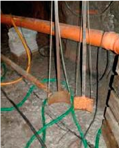
Figure 3-9. Tools for inducing core breakage, double steel plates (before being expanded using hydraulics), (from Mærsk Hansen and Staub 2004).
