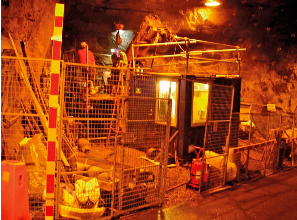
Figure 3-22. The fenced-in drill site for the TRUE-1 overcoring activity, drill rig in position for overcoring of KXTT3.
