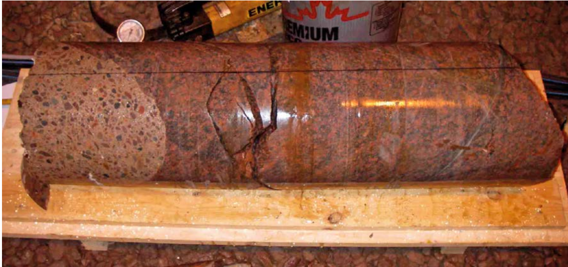
Figure 3-20. The first core pieces from borehole KXTT3 in core box at drill site, where preliminary core logging, orientation and photographing was performed. Top of core to the left, concrete slab visible, black line marks vertical down of core. Length of core is approximately 0.0–0.74 m.
