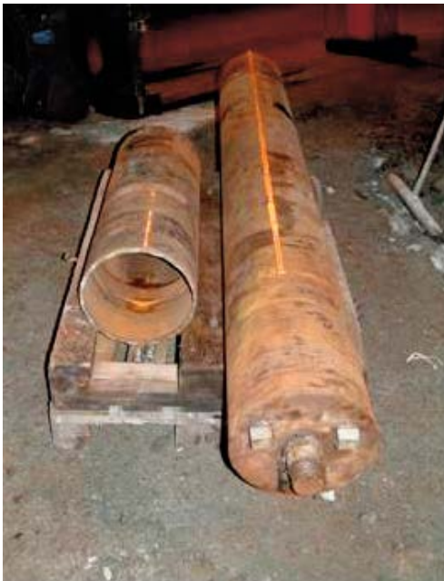
Figure 3-8. 300 mm Core barrels of 76 cm and 225 cm core length, respectively (from Mærsk Hansen and Staub 2004).
