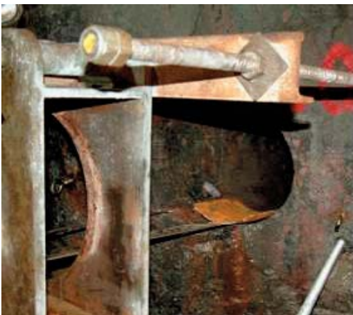
Figure 3-10. Insertion of tool for core breakage, sliding below core (from Mærsk Hansen and Staub 2004).
