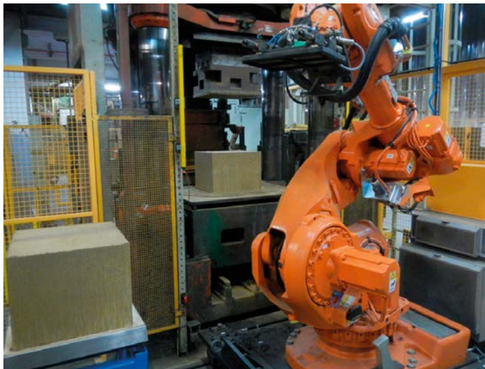
Figure 7-5. Press and industrial robot used to produce the blocks.
