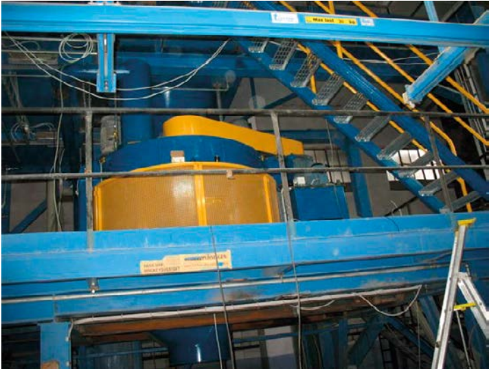
Figure 7-4. Eirich mixer used to mix the material.
