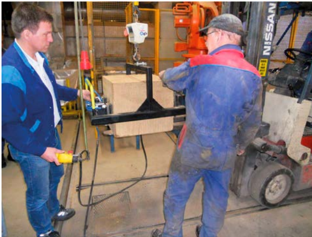
Figure 7-1. Manual handling of backfill blocks.
