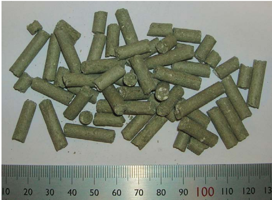
Figure 4-2. Bentonite pellets produced by extrusion.
