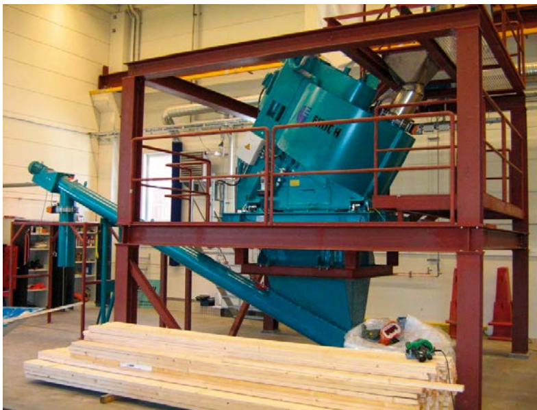
Figure 5-2. Eirich mixer used at Äspö.
