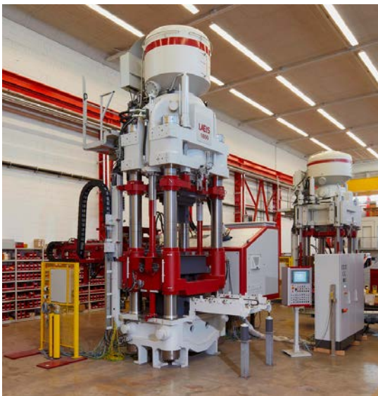
Figure 5-3. A HPF 1600 press from Laeis.
