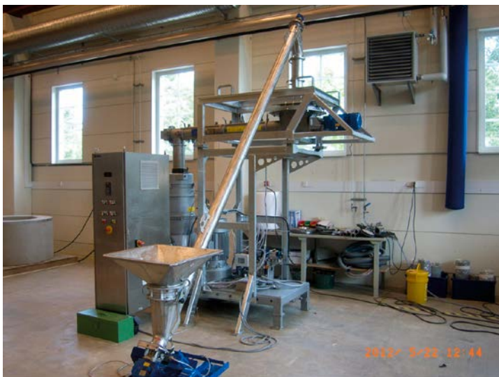
Figure 5-5. Pellet press for extruded pellets used for test production at Äspö.
