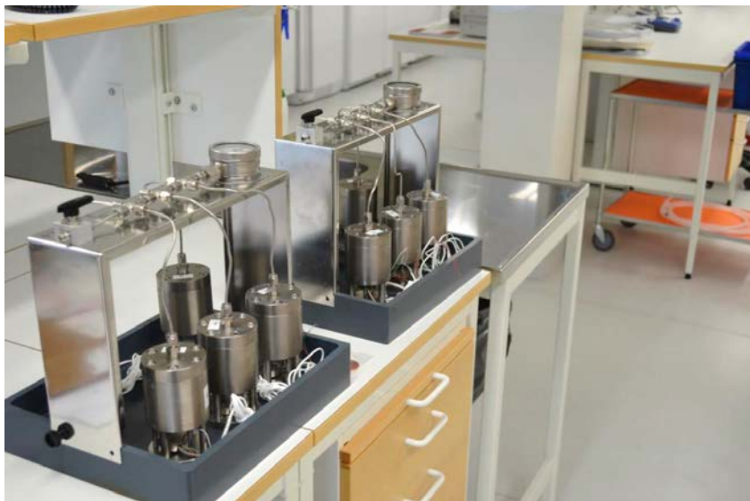
Figure 2-3. Water saturation system with ten mounted test cells positioned upside down.
