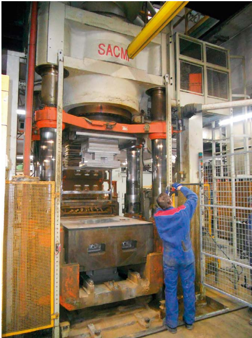
Figure 4-2. Photo showing the new mould after installation in the SACMI press.
