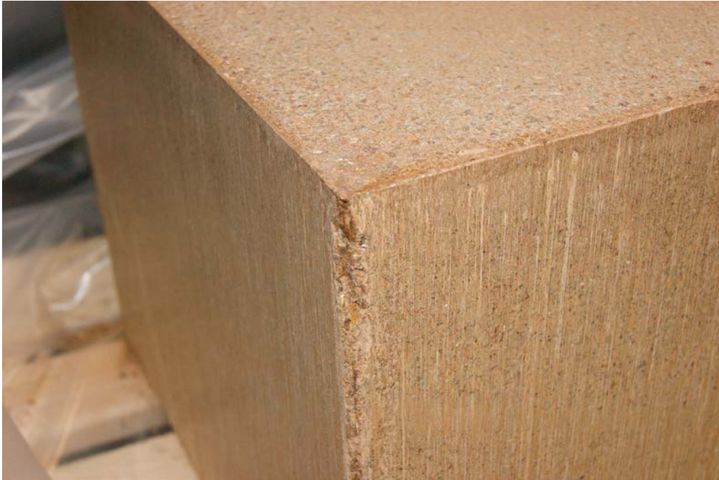
Figure 5-9. Close up showing one of the vertical edges which still were very fragile.
