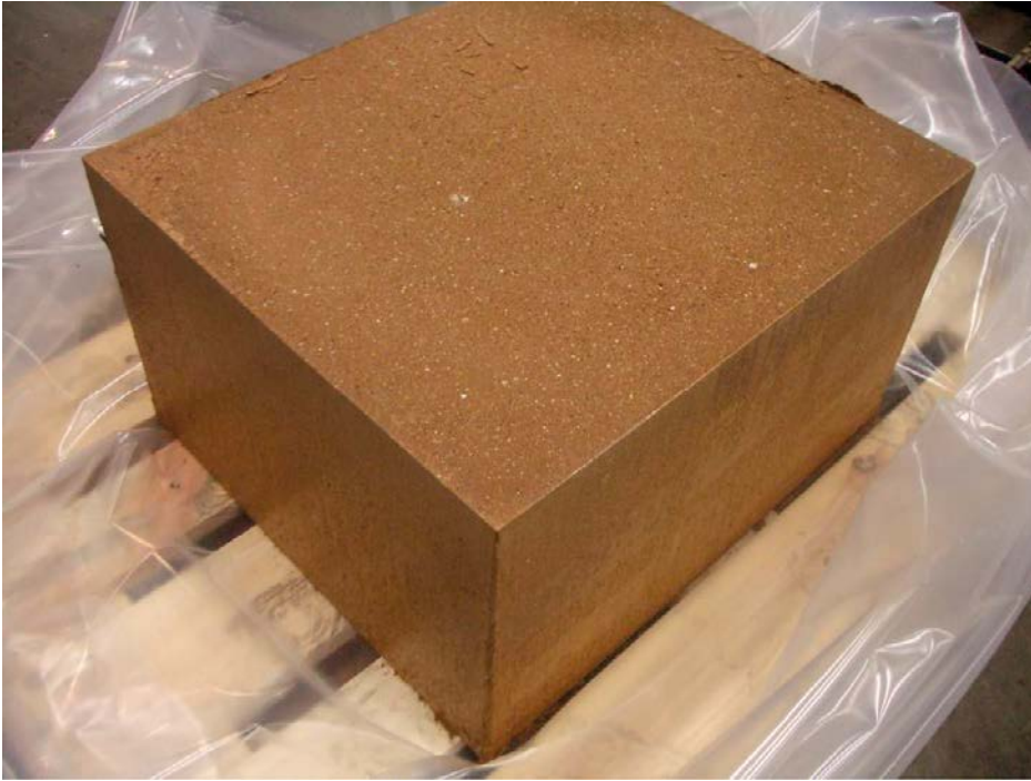
Figure 5-19. Photo showing an Asha 2010 block manufactured with the crushed material and with a water content of 20%.
