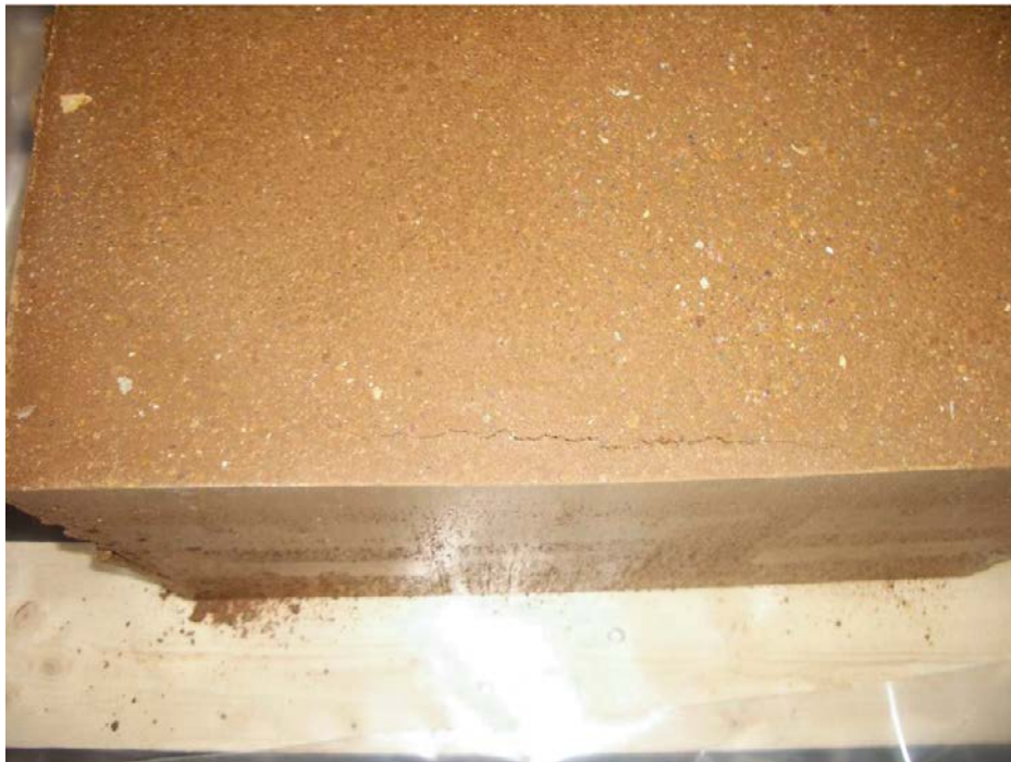
Figure 5-18. Photo showing an example of the crack that occurred in the blocks with the highest water content, 24%.
