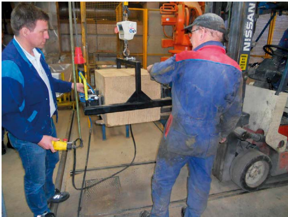
Figure 4-4. Photo showing the special lifting equipment used during the block testing.
