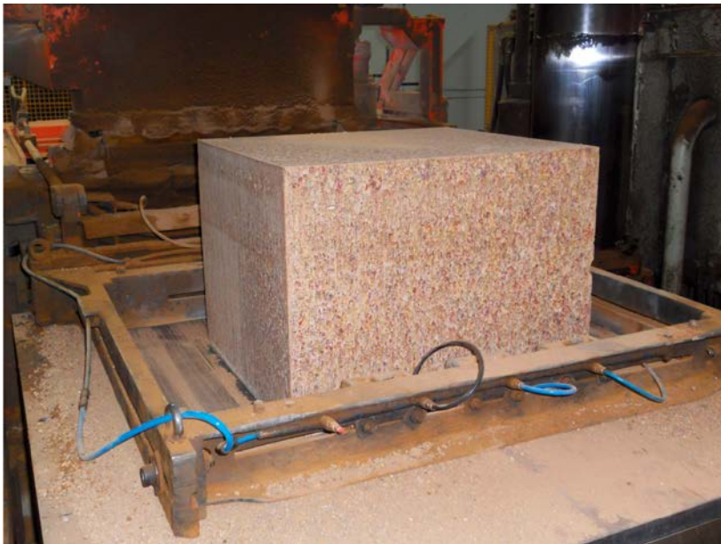
Figure 5-4. Photo showing one of the first blocks compacted in the new mould.
