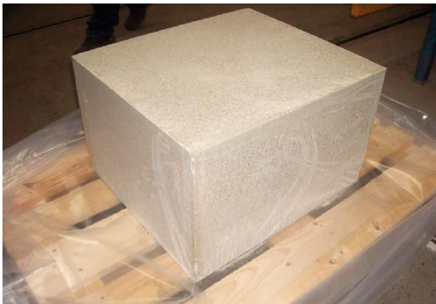
Figure 5-21. One of the blocks manufactured with MX-80. The block quality was high even if the four vertical edges were somewhat fragile.
