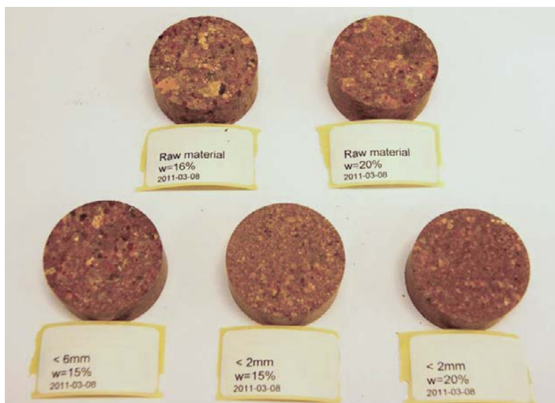
Figure 3-7. Photo showing the samples after compaction.
