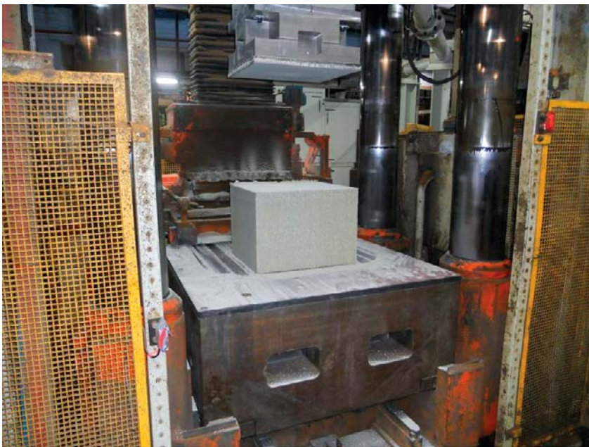
Figure 5-7. Photo showing one IBECO block with rather good quality directly after compaction.
