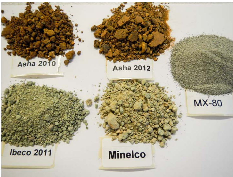
Figure 2-1. Photo showing the different materials used in the tests.
