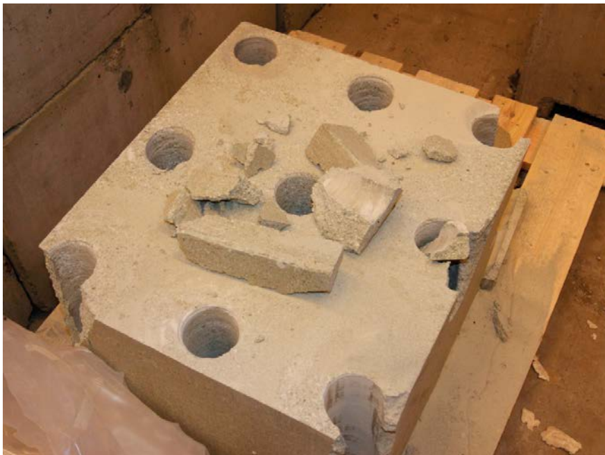
Figure 4-8. Photo showing a block after sampling.
