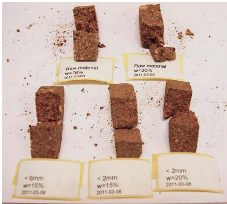
Figure 3-9. Photo showing the samples after a rough break of the samples.
