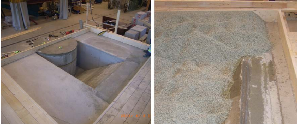
Figure 5-5. Left: Upper part of a deposition hole included the bevel was built in concrete. Right: Water flow applied as a “fracture” at the edge of the bevel. (Johnsson 2011).
