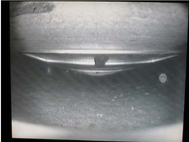
Figure 5-4. The bottom of a distance block seen with the camera in the front of the sliding plate after deposition. A small dark spot in the upper left corner probably comes from splashing.
