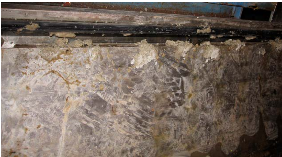
Figure 5-6. The lifting pallet after deposition of the Supercontainer. Wetted bentonite was left on the pallet.
