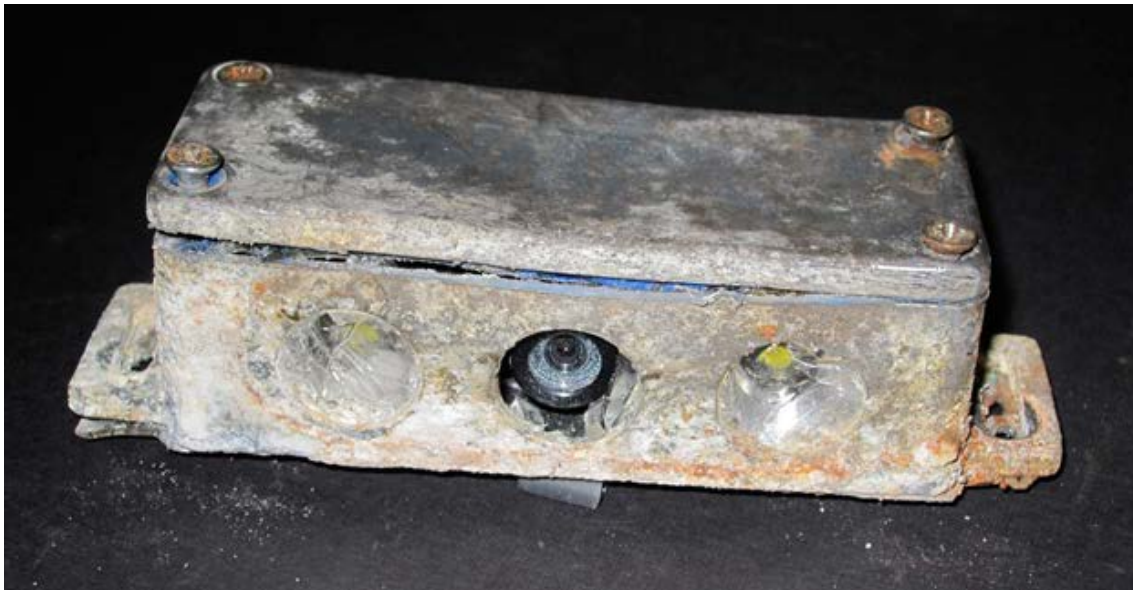
Figure 3-14. The camera unit with two power LED's for lighting and a camera in the middle. Protective glass cracked and fallen apart.
