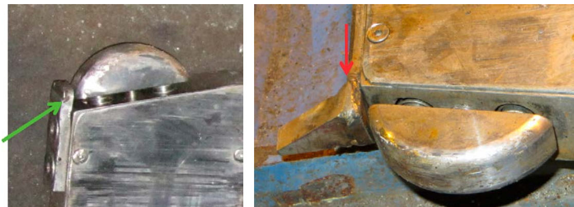
Figure 3-6. To the left the old collision sensor protection consisting of a plate. To the right the new collision sensor protection guiding the sliding plate down.
