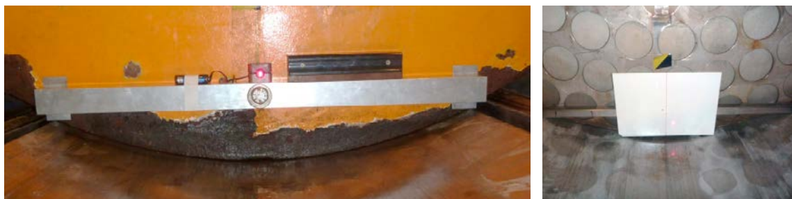
Figure 3-19. The calibration tool developed for aligning the lifting pallet with the machine. The ruler against the shield on the left and the target plate in front of the Supercontainer on the right.
