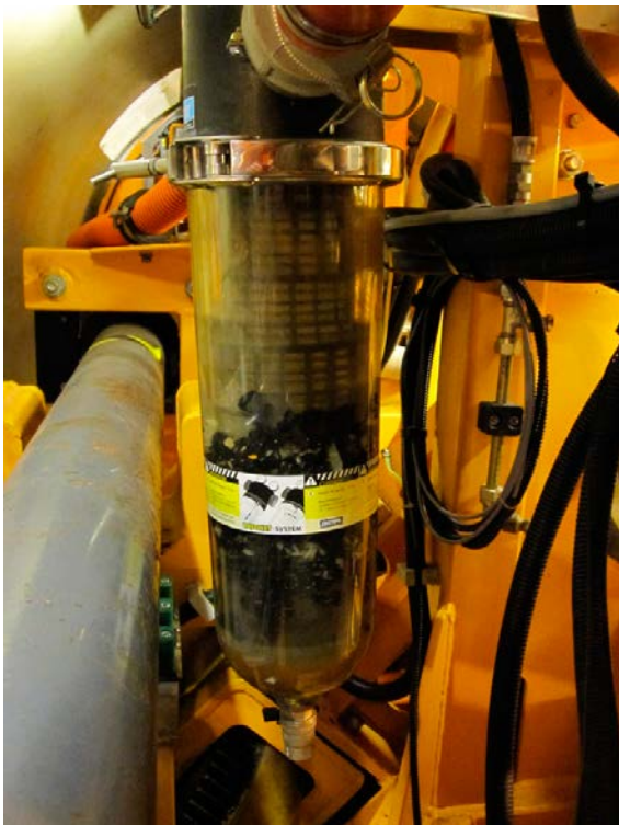
Figure 3-7 . Black chips from the guiding edges of the sliding plate in the water filter.
