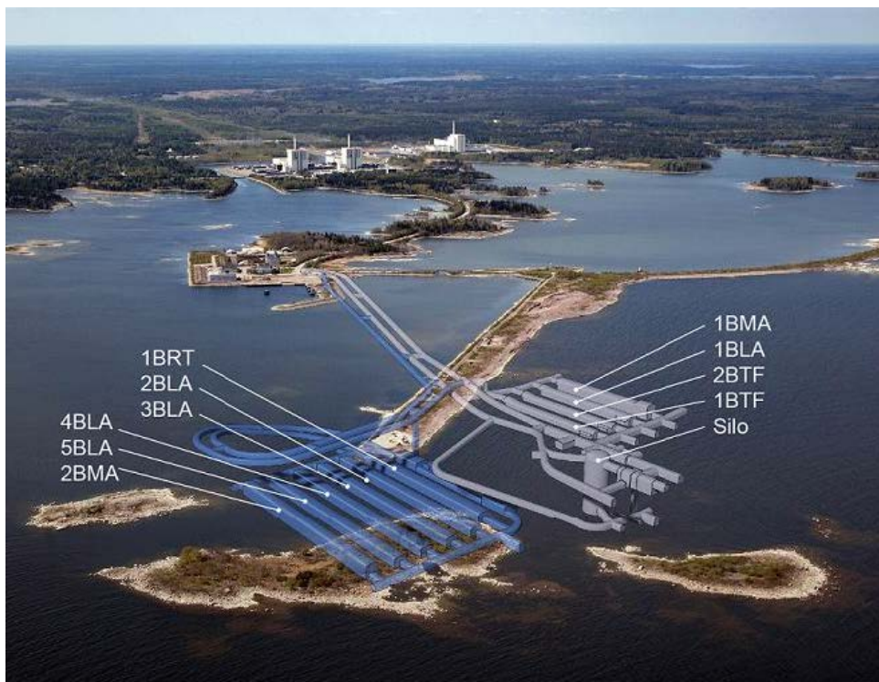
Figure 1-1. The proposed extension of the SFR repository. The present SFR repository is located to the right (light grey colour) while the planned new tunnel system is shown to the left (light blue colour). The existing facility is situated about 60- 140 m below the seabed of the Baltic Sea, while the extension is proposed to reach c. 120 m below sea level.
