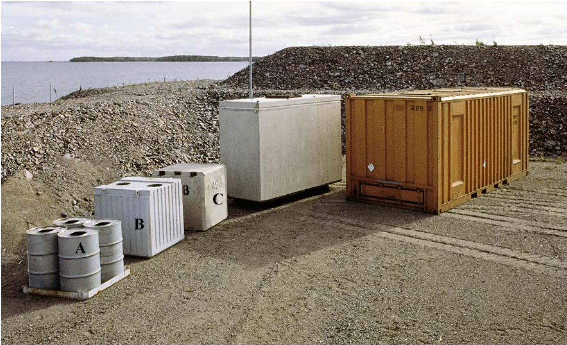
Figure 2-4. Illustration of the various types of waste packages stored in the SFR repository. The picture shows the steel drums (A), the steel mould (B) and the concrete mould (C) used for storing waste in the BMA vault.
