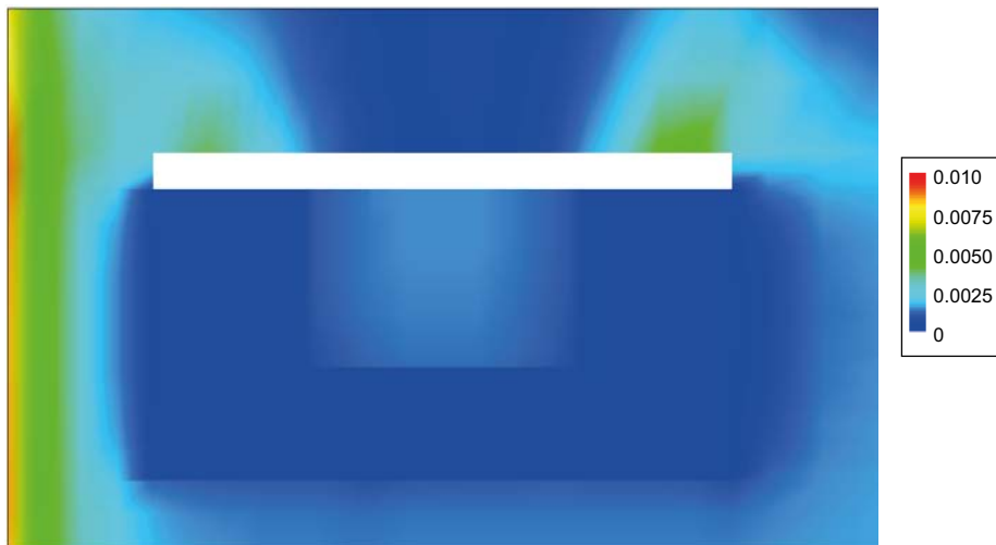
Figure 7-46. Calcite precipitation due to the reaction between calcium leached from the concrete and carbonate in the inflowing groundwater. Units are \text{kmol/m}^3 of pore water. Blue colour denotes that no calcite is present, red colour denotes the maximum precipitation of 0.01 \text{ kmol/m}^3 of pore water.
