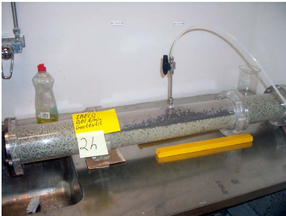
Figure 3-1. Photo showing the test equipment used in order to study the function of geotextiles as water distributor.
