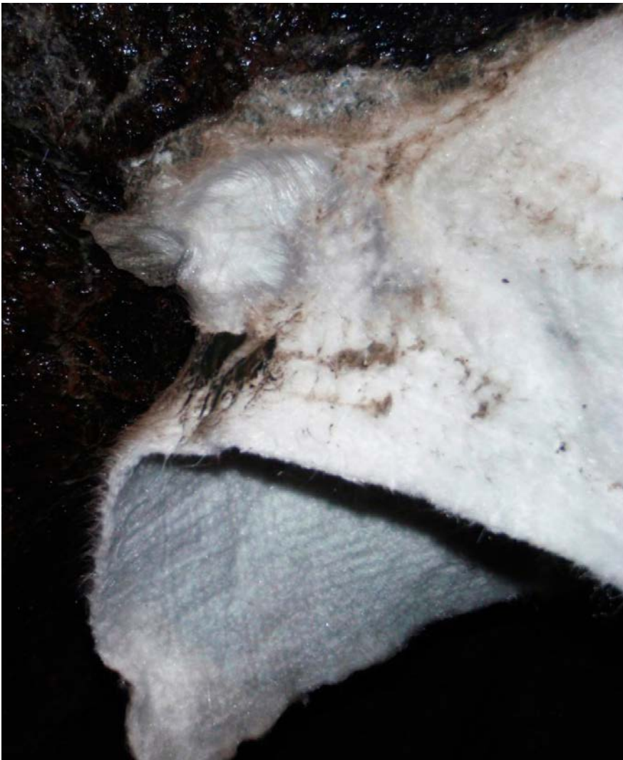
Figure 5-7. The attachment was stronger than the glass fibre fabric.
