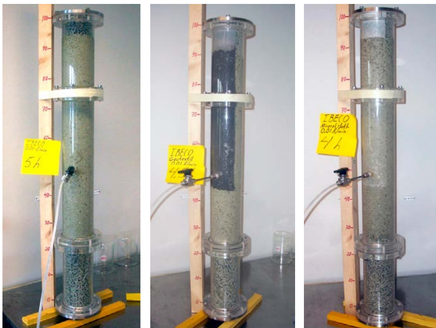
Figure 3-5. Photos taken after 4 to 5 hours test time. The left photo shows the reference test, the middle photo shows the test performed with standard geotextile and the right photo shows the test performed with fibre glass fabric I.
