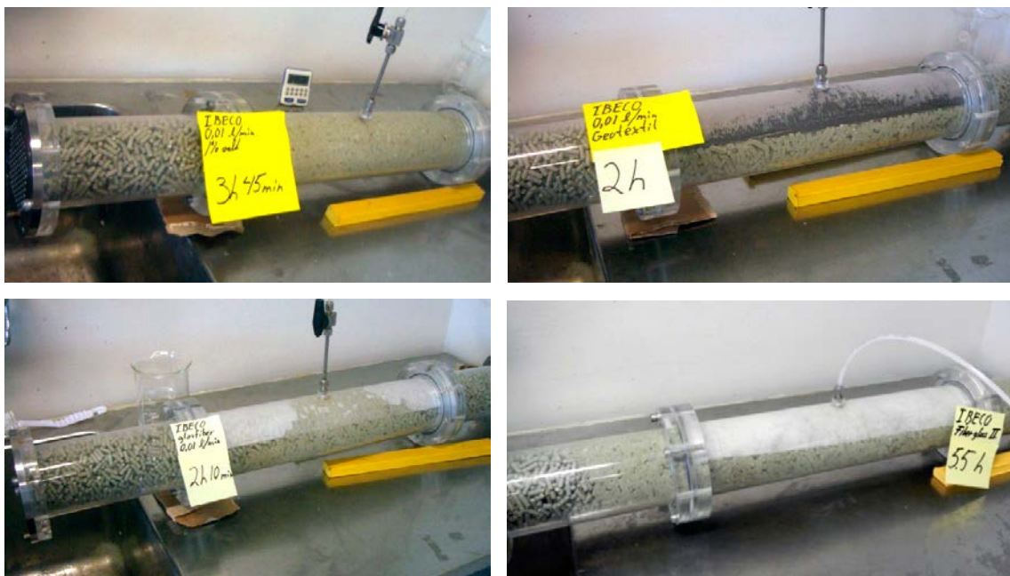
Figure 3-7. Photos showing the tests performed in horizontal direction with different fabrics. Upper left: Reference test Upper right: Test with geotextile of standard type Lower left: Test with fibre glass fabric Lower right: Test with thicker fibre glass fabric.
