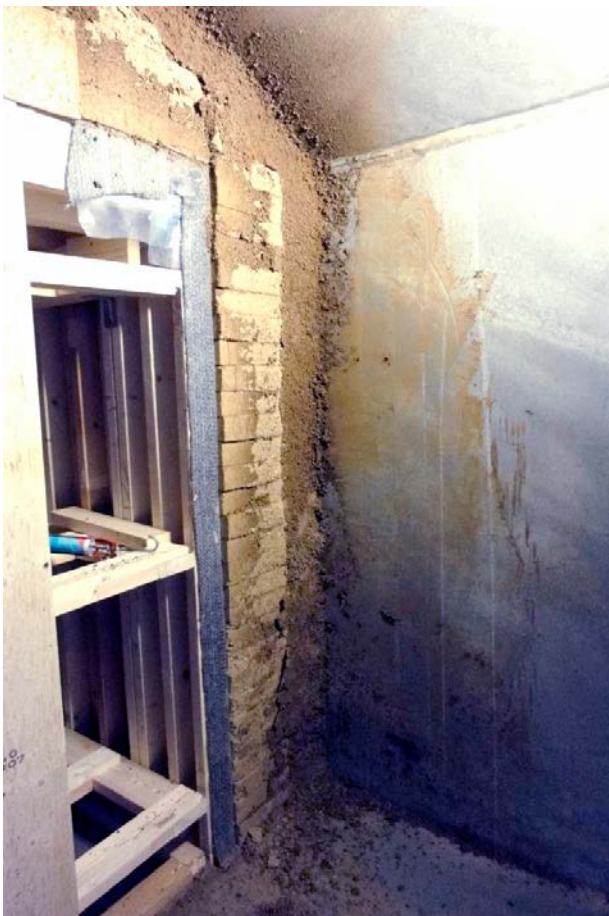
Figure 4-3. The backfill front during a test.
