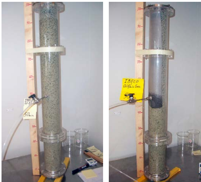
Figure 3-3. Photos taken after 50 minutes test time. The left photo shows the reference test and the right shows the test equipped with geotextile.
