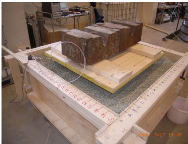
Figure 2-1. Arrangement for studying wetting of pellet fills. Water is pumped from a hole drilled through the rock block located under the fill that is covered by the wooden plate. Notice the coordinate system for describing the position of the samples taken.
