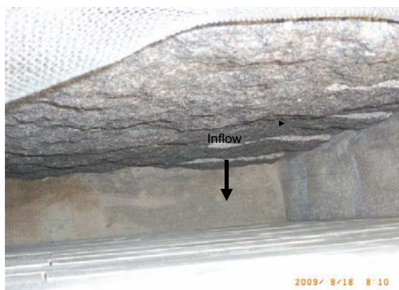
Figure 2-2. View of the space between rock and block wall to be filled with pellets in all tests except one (V4). In test V4 the pellets were confined by a net supported by a wooden construction.
