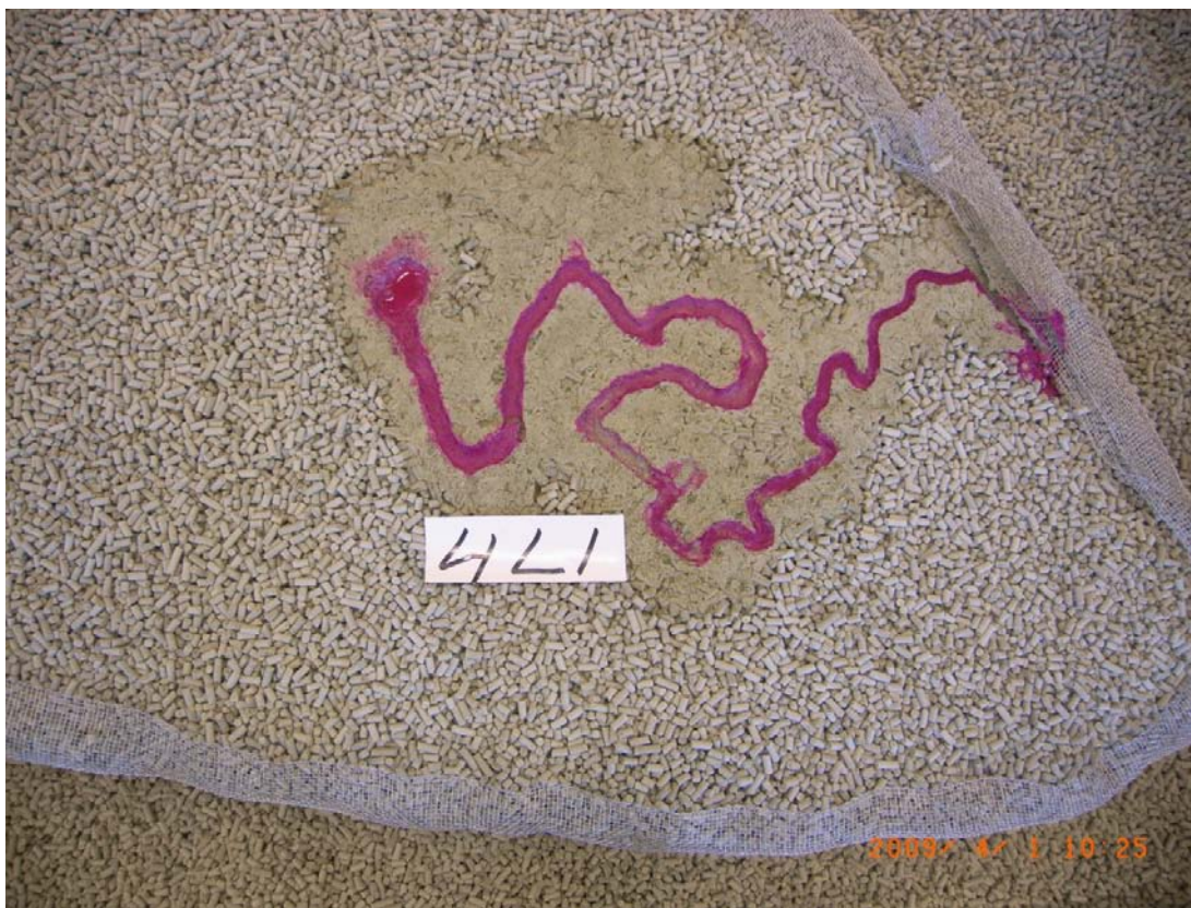
Figure 2-10. Migration of the water content in the three layers in test H4 with an inflow rate of 0.1 l/min. Upper: Distribution of the water content indicating formation of a plume that widened upwards and ultimately gave a channel through which all water flowed, eroding the pellet fill. Lower: Photo of upper surface with meandering water expelled from the steep channel (Photo by Hedin).
