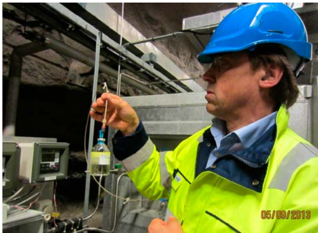
Figure 2-1. The inoculation process in VLJ repository to anaerobic butyl rubber-stopped bottles using syringes.
