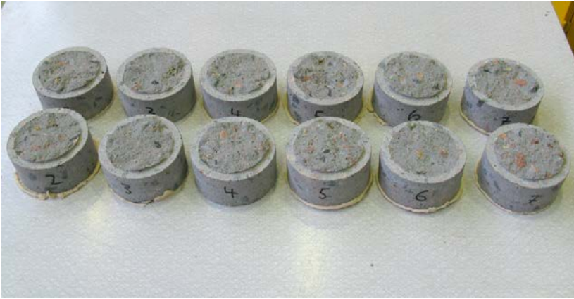
Figure B-7. Photo of the direct tensile tests specimens (DTT-C-#) after testing.
