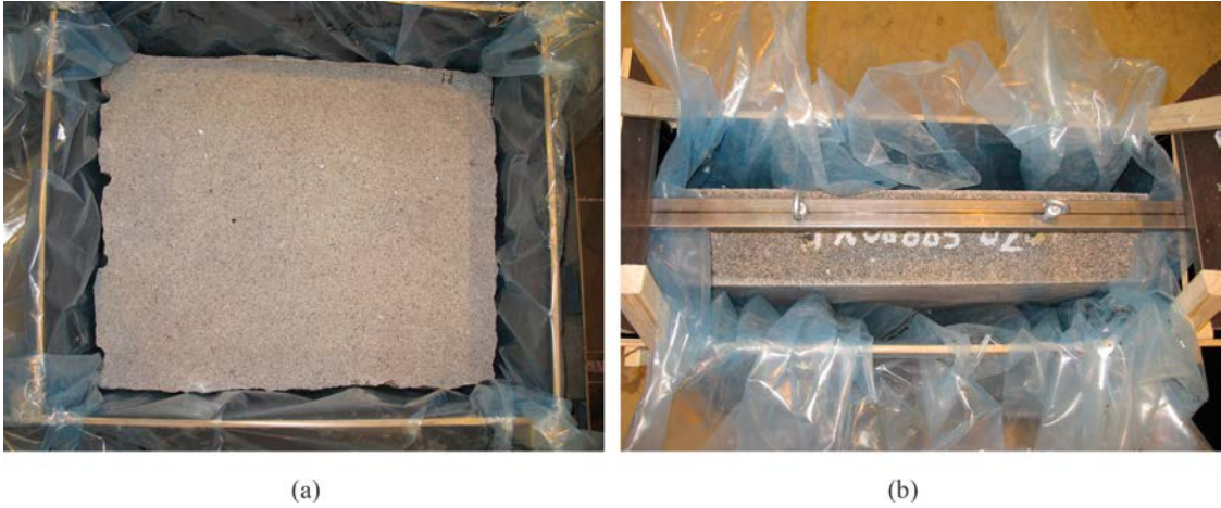
Figure 2-3. Photo of rock panels placed in the in the moulds before casting. The casting was performed a) against a horizontal surface and b) against vertical surfaces.
