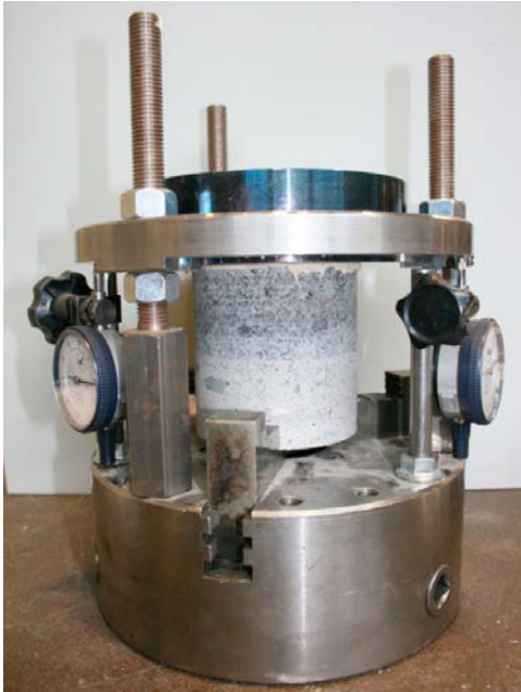
Figure 3-3. Photo of the “glue device” (with lower loading platen in upper part of picture).
