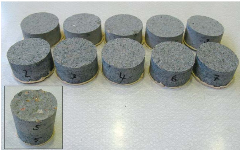
Figure C-7. Photo of the direct tensile tests on rock-concrete interface specimens (DTT-RCI-#) after testing.
