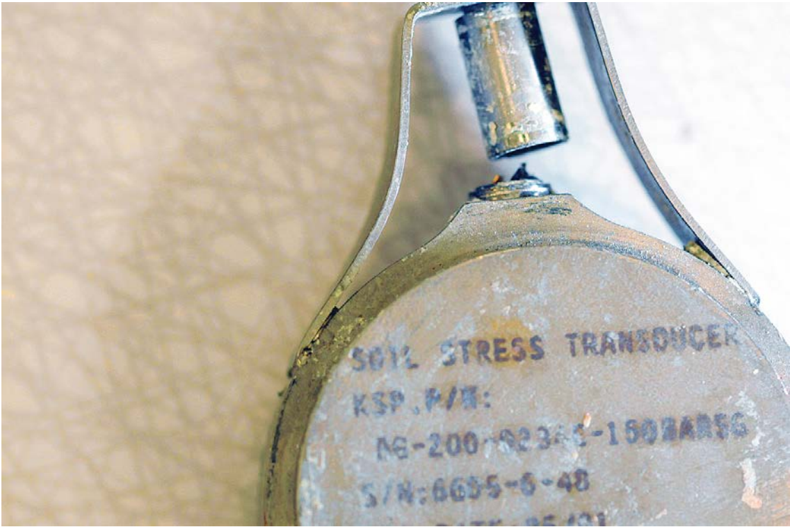
Figure 5-7. Sensor 6655-6-48 Kulite; broken connection at housing.
