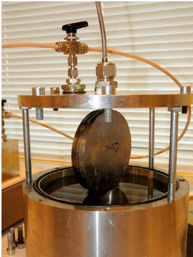
Figure 3-1. Test cell with a total pressure sensor before immersion into water.
