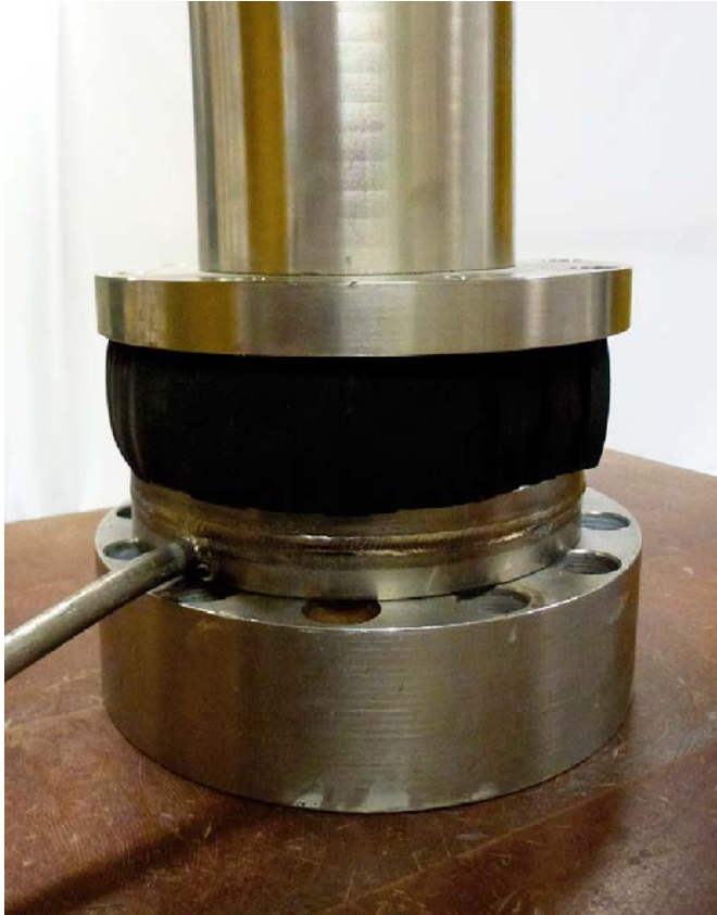
Figure 3-2. Total pressure sensor tested with mechanical force and a rubber pad.
