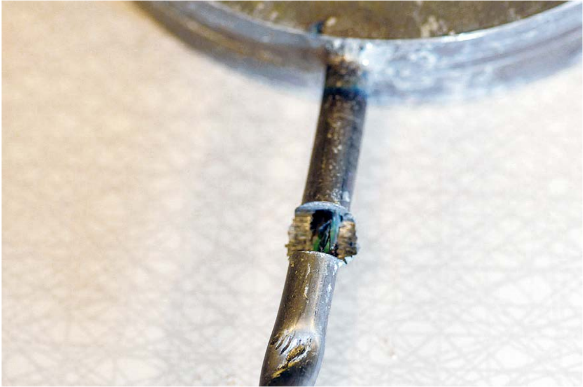
Figure 5-4. Sensor 62293, PB 613 Dismantling damage caused by core drilling for the buffer sampling.
