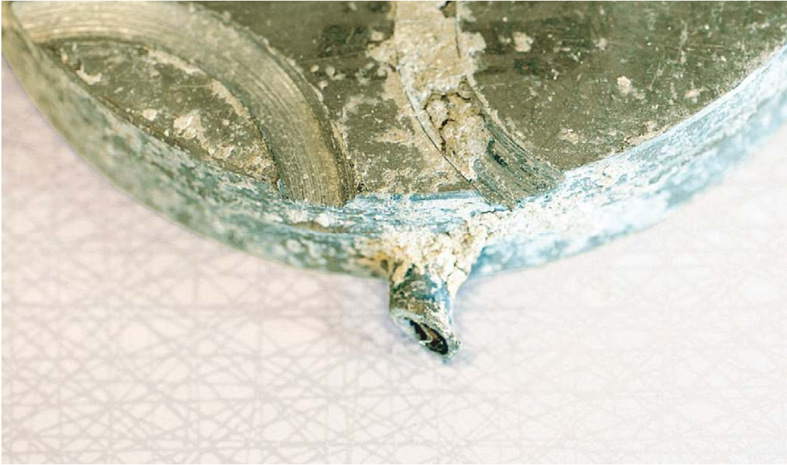
Figure 5-2. Sensor 62281, PB 527 Dismantling damage caused by core drilling for the buffer sampling.
