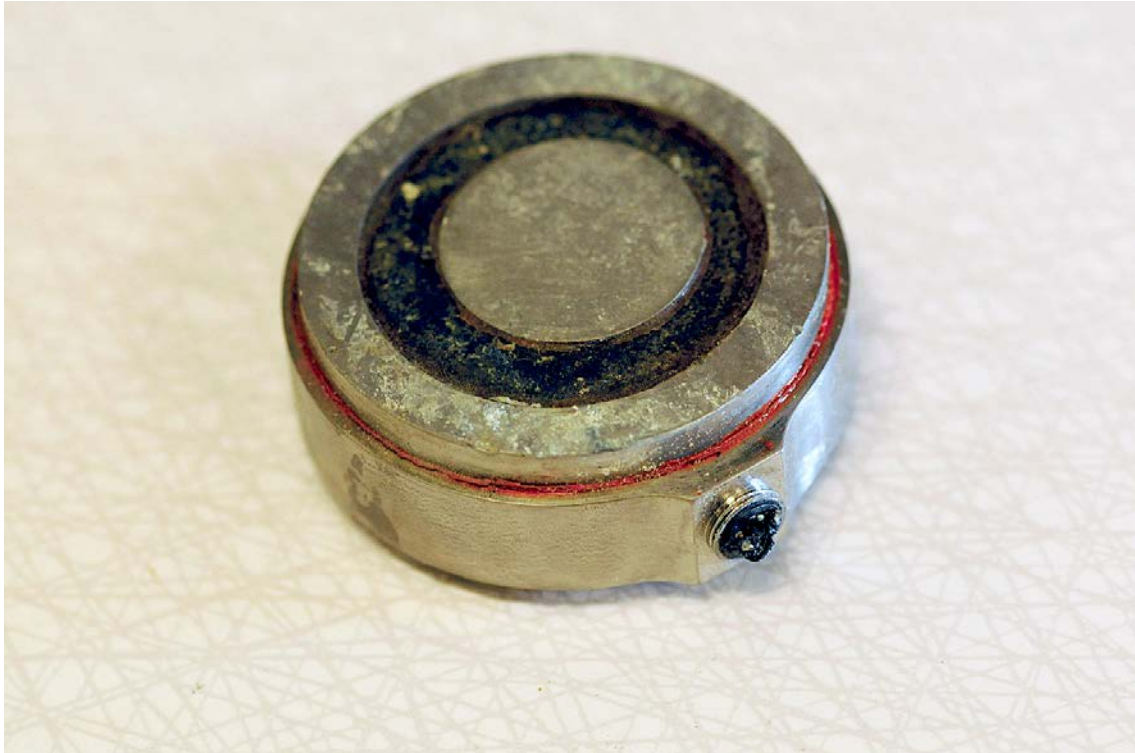
Figure 5-10. Sensor 6605-6-31 Kulite; broken connection at housing, probable resin cast in Figure 5-11.
