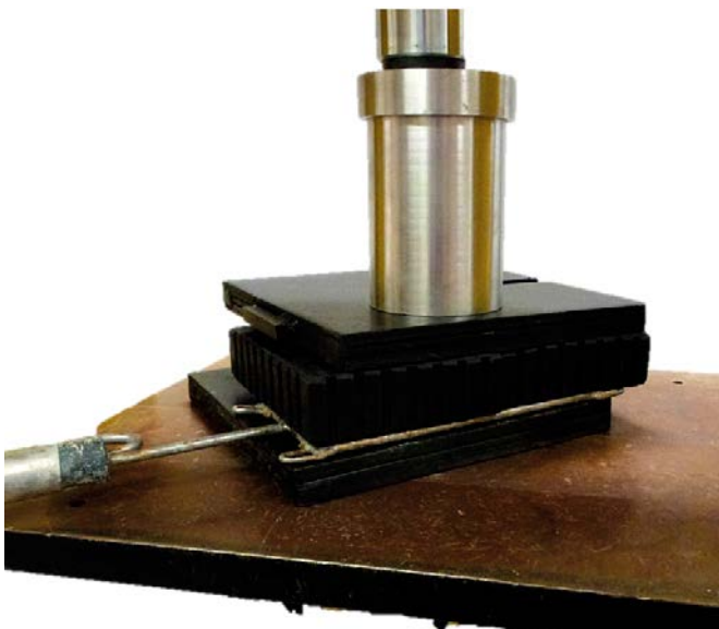
Figure 3-3. Total pressure cell under testing, the cell was installed in the backfill.
