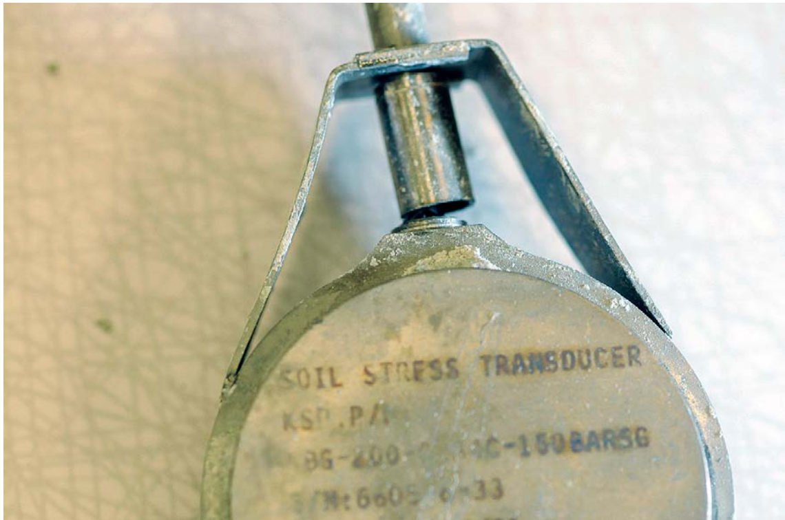
Figure 5-8. Sensor 6605-6-33 Kulite; broken connection at housing.
