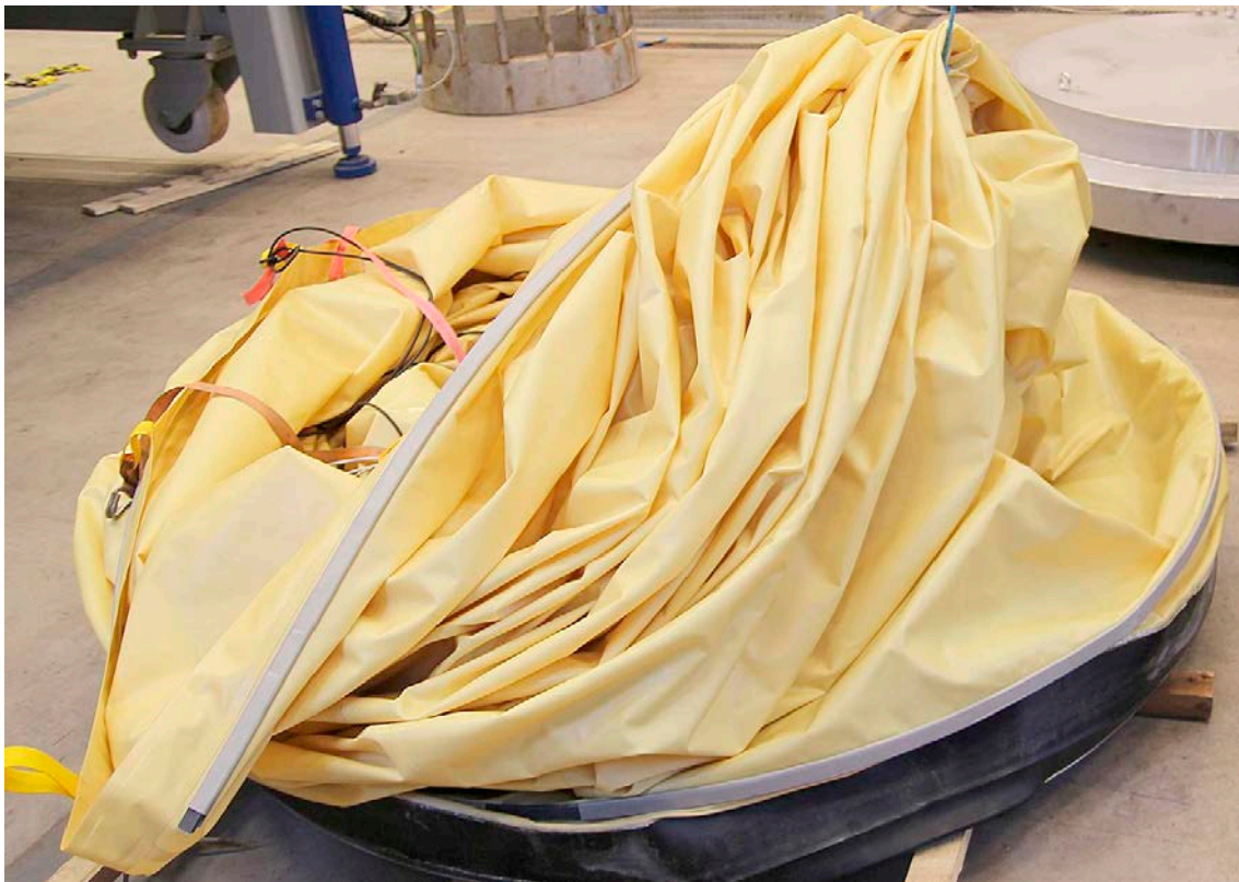
Figure 4-1. Photo of the assembled bottom plate and buffer protection sheet in the bentonite laboratory at Äspö.
