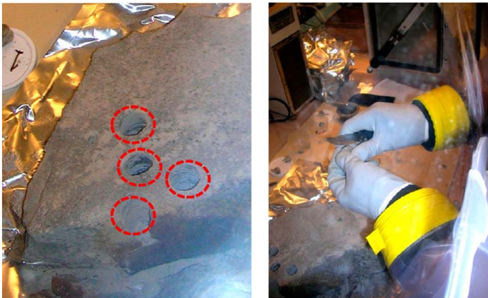
Figure 1-14. Sampling for Mössbauer analysis in glove box. (TR03_250_C31, TR03_250_C33, TR03_250_C35 and TR03_250_C39)
