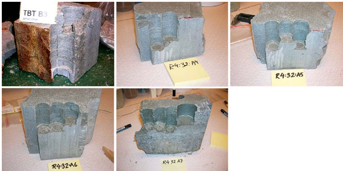
Figure 1-11. Sampling for hydro-mechanical analyses. Specimens from Ring 4 in 32° direction. From B level close to heater (upper left), and from A level (all other photos);
