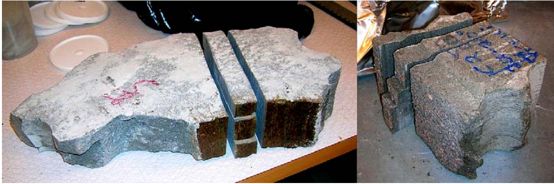
Figure 1-13. Sampling for XANES and electron microscopy: inner piece from Ring 4 in 330° direction and B level (left) and outer piece from Cylinder 2 in 212° direction and B level (right).
