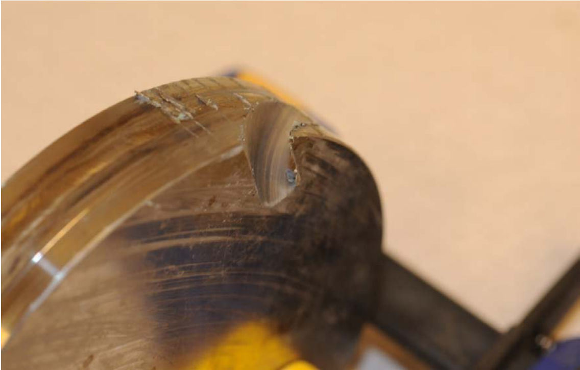
Figure B-7. Sensor Geokon 70042 drill damage.
