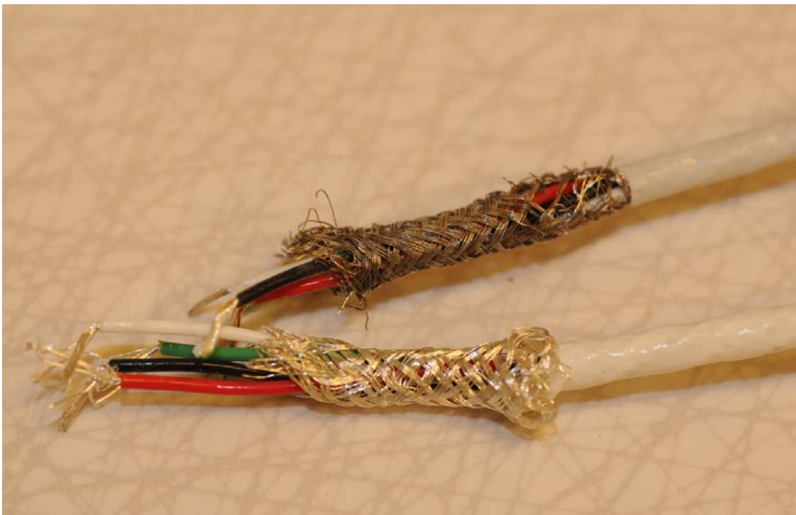
Figure B-10. Sensor cables, the upper showing corrosion in the shield from water. 70039, 70055.
