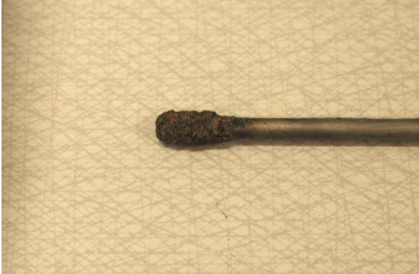
Figure B-13. Filter tip from injection point AS205 with precipitates.
