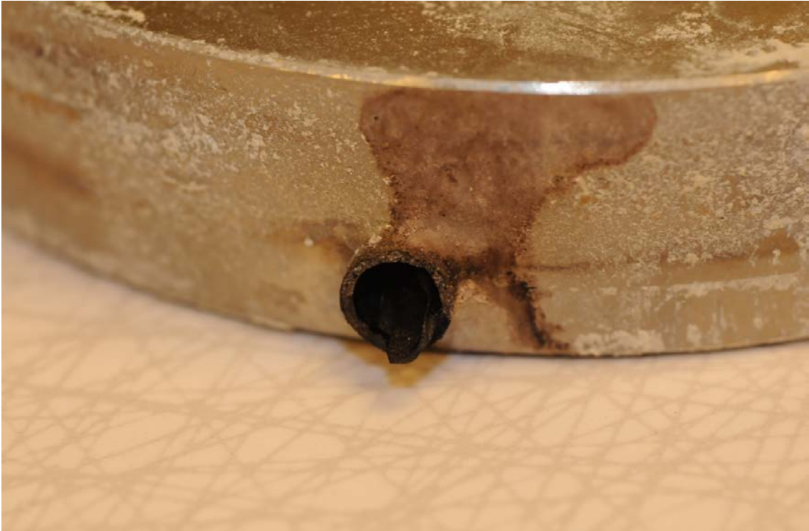
Figure B-8. Sensor 70054, broken in the weld to the housing.
