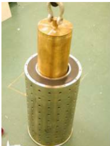
Figure 4-23. Model canister being lowered into support cage containing bentonite pellets in annulus.
