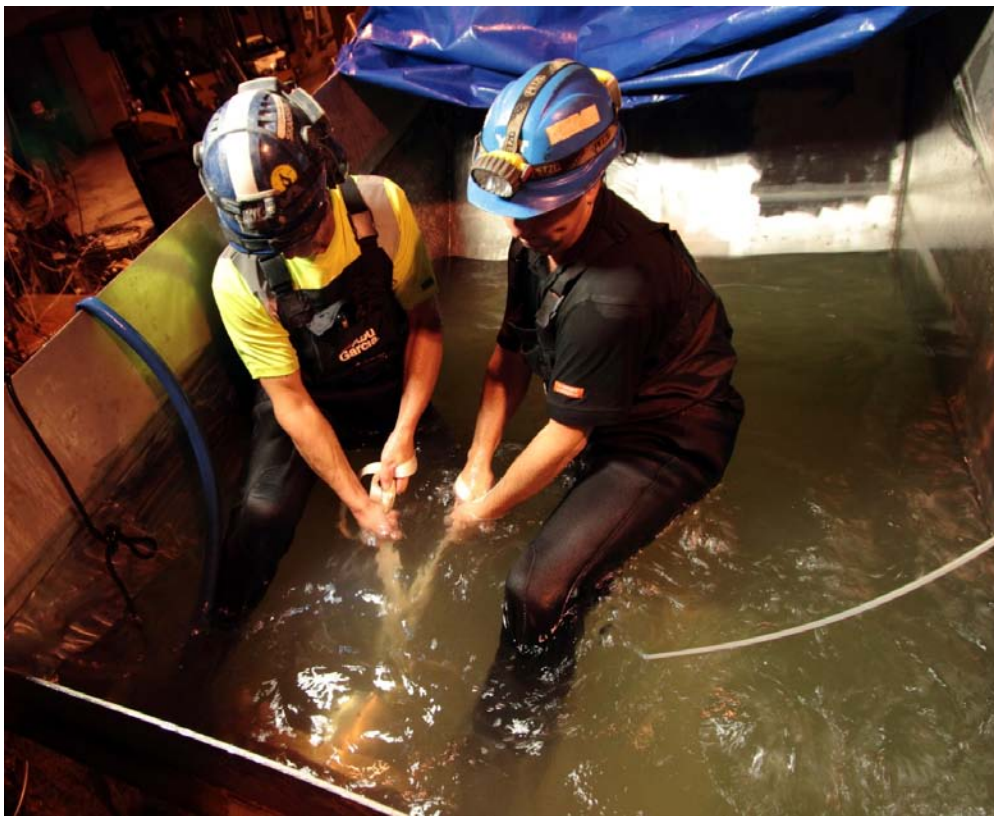
Figure 4-24. Stefan Grandin Svårdh and Jonas Hallberg pulling out the steel cage from the KA3386A04 bore hole.
