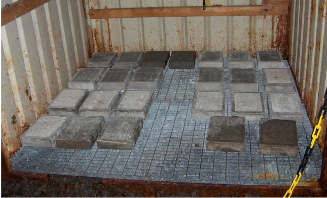
Figure 4-30. Container in Äspö HRL with samples corrosion tests.
