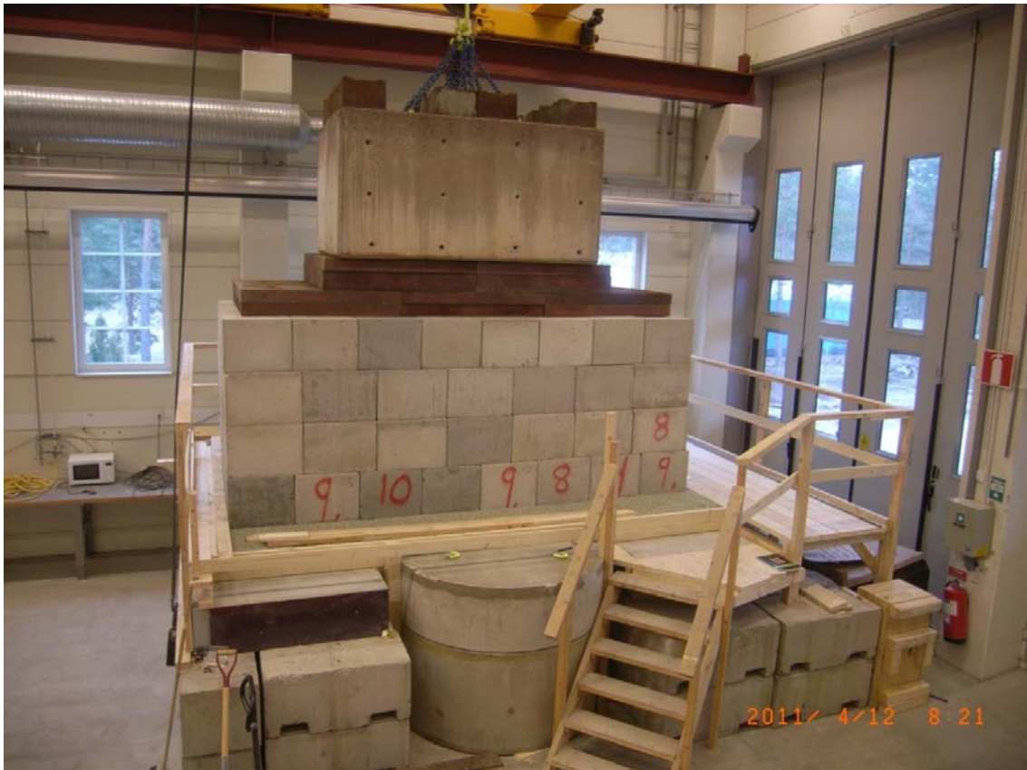
Figure 6-5. Block stacking on the upper part of the deposition hole and bevel.
