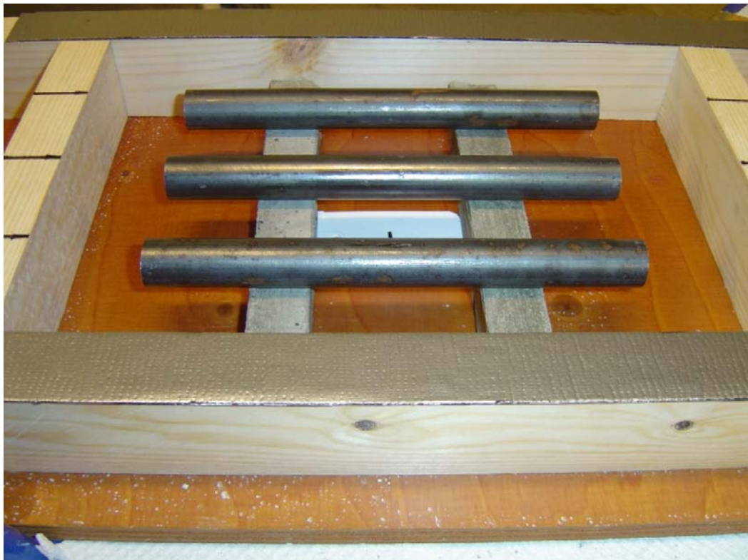
Figure 4-29. Mould and steel bars on supports before casting.
