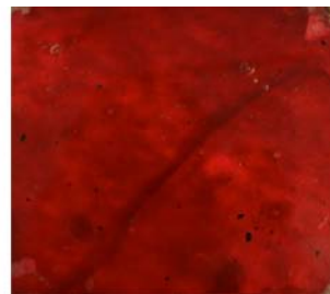
Figure 3-8. Picture of Rock fracture from Äspö left and the two cast sides fitted together with red dye between them.
