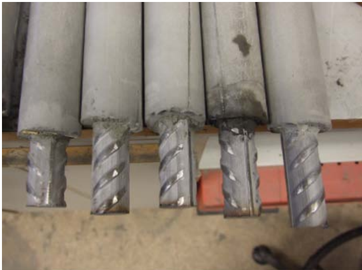
Figure 7-11. Grouted rock bolts of stainless steel.
