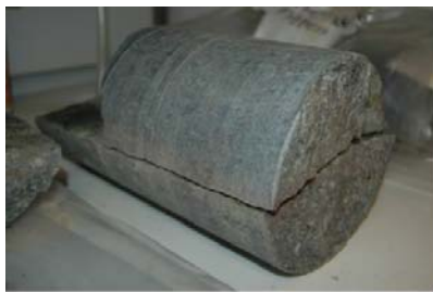
Figure 3-8. Picture of Rock fracture from Äspö left and the two cast sides fitted together with red dye between them.
