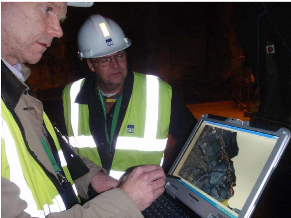
Figure 2-4. TASS-tunnel. A first test of the RoCS mapping system (a prototype) in tunnel environment. The mapping is taken place directly on the laptop screen.
