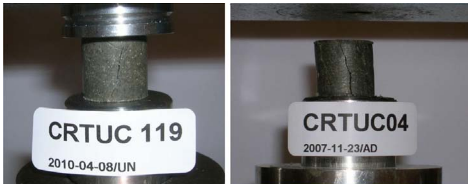
Figure A1-1. Specimens CRTUC119 and CRTUC04 from the innermost part of the buffer with dry densities of 1,530 \text{ kg/m}^3 and 1,600 \text{ kg/m}^3 , respectively.
