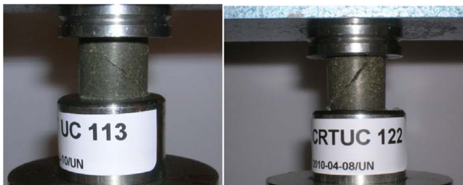
Figure A1-2. Reference specimens CRTUC113 and CRTUC122 with dry densities 1,540 \text{ kg/m}^3 and 1,620 \text{ kg/m}^3 , respectively.
