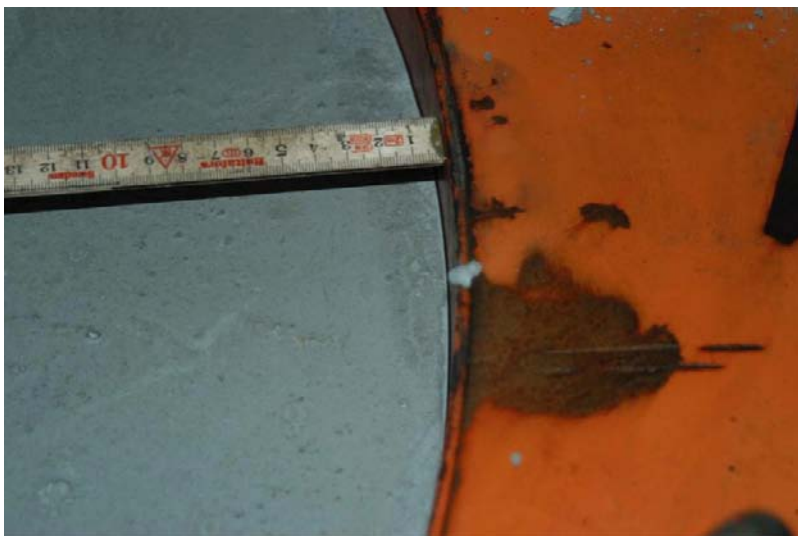
Figure 3-12. Experimental gap between the concrete and the steel mould.
