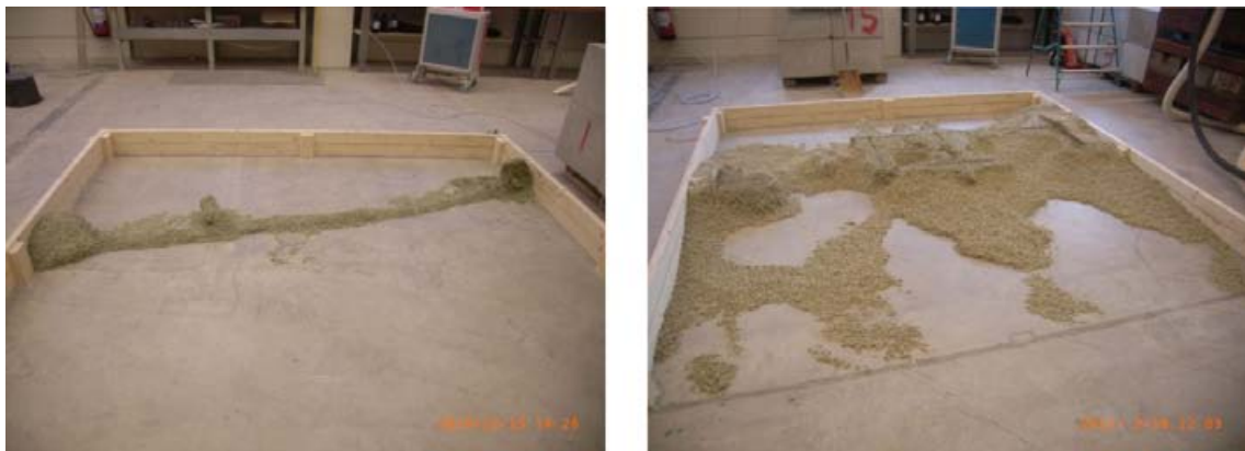
Figure 2-8. The remaining pellets after the block stack and dry pellets removed. Left, test 5 and right test 6.
