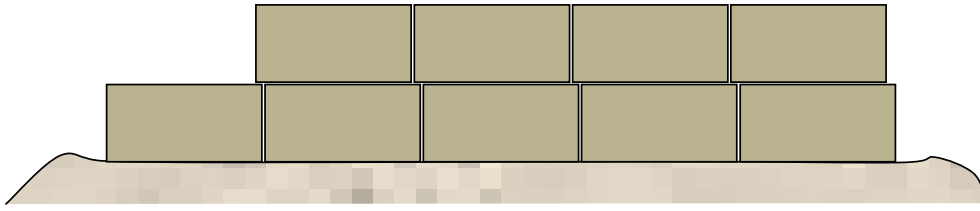
Figure 2-2. Stacking method used in test 1–2.
