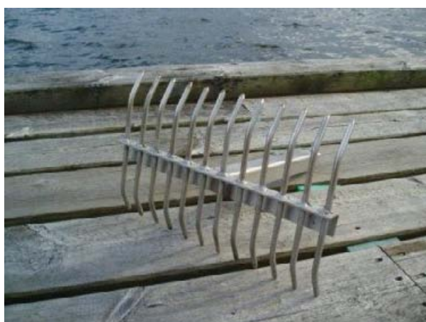
Figure 2-2. A plant rake, B Luther, a stainless steel rake on a rope used for sampling of macrophytes.
