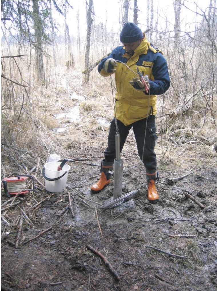
Figure 4-2. Initiation of the rising-head test in groundwater monitoring well SFM0067, installed in soil. The evaluation of slug tests is facilitated if the data demonstrate a distinct change of the water-pressure head at the initiation of the tests. This is particularly important for wells where the screens are installed in permeable soil layers, as the subsequent transient response of the water level is relatively fast in such wells. In order to achieve such a distinct change of the water-pressure head, the slug must be raised from the well as quickly as possible when the test is initiated.
