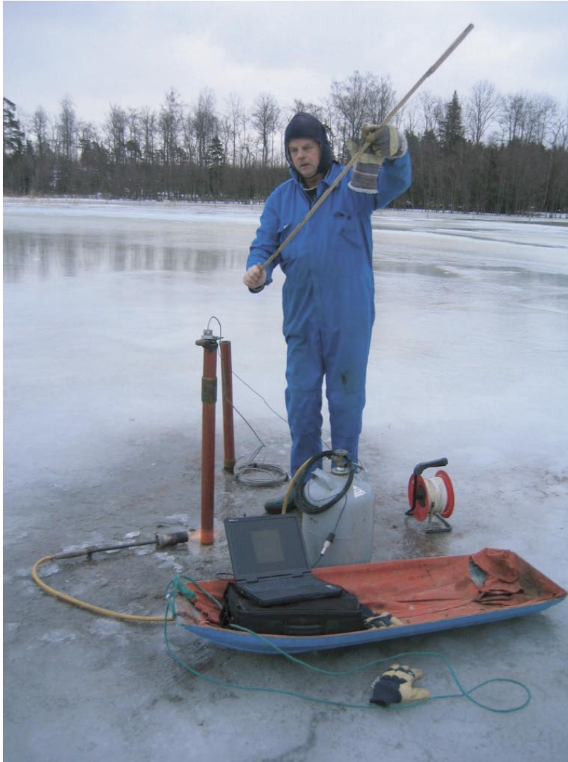
Figure 4-1. Falling-head test in groundwater monitoring well SFM0065, installed in soil below open water. The slug (connected to a stainless-steel wire) is lowered into the well. The Diver®, hanging at a known depth in the well, is connected by the black cable to the portable PC on the sledge. A spanner wrench is utilized as wire stop. All wells installed in soil below open water (SFM0022, 0062-63, and 0065) were tested when the lakes were ice covered. As a consequence, the frozen water in the near-surface section of the stand pipe had to be melted using a LPG burner prior to initiation of the slug tests in these wells.
