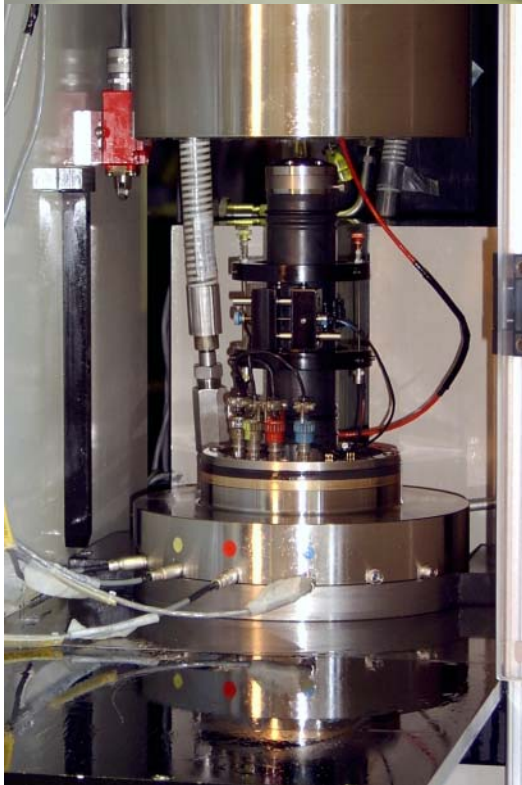
Figure 3-1. Left: Digital controller unit, pressure cabinet with cell pressure intensifier and oil reservoir inside, load frame with closed cell (pressure vessel). Right: Bottom of the cell is lowered. The specimen is instrumented and ready for inserting in the cell.
