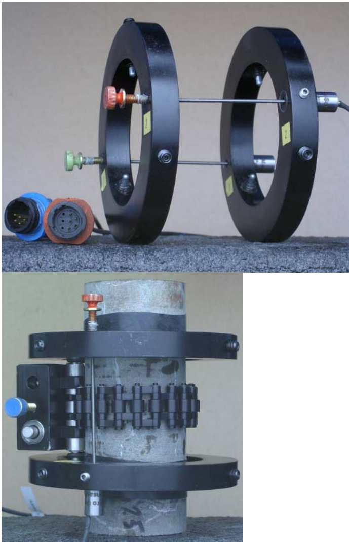
Figure 3-2. Left: Rings and LVDTs for local axial deformation measurement. Right: Specimen with two rubber bands. Devices for local axial and circumferential deformation measurements attached on the specimen.
