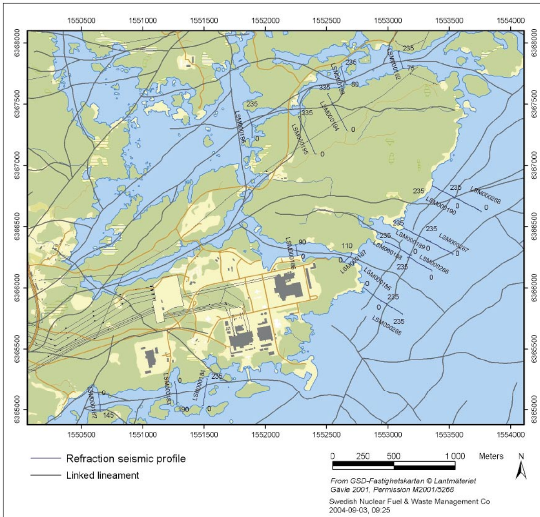
Figure 1-1. Location of refraction seismic profiles in the sea outside Simpevarp and Ävrö and on Ävrö. Lineaments presented are linked lineaments interpreted from air photos and helicopter airborne geophysics /3/.
