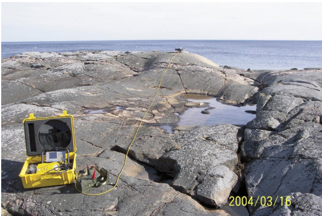
Figure 3-3. A choke ring antenna with the new type Trimble R7 receiver at site OKG in March 2004.
