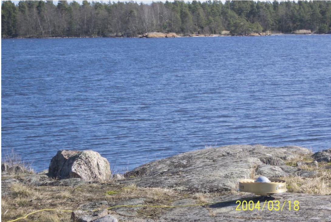
Figure 3-2. A choke ring antenna at site Åspö in March 2004.
