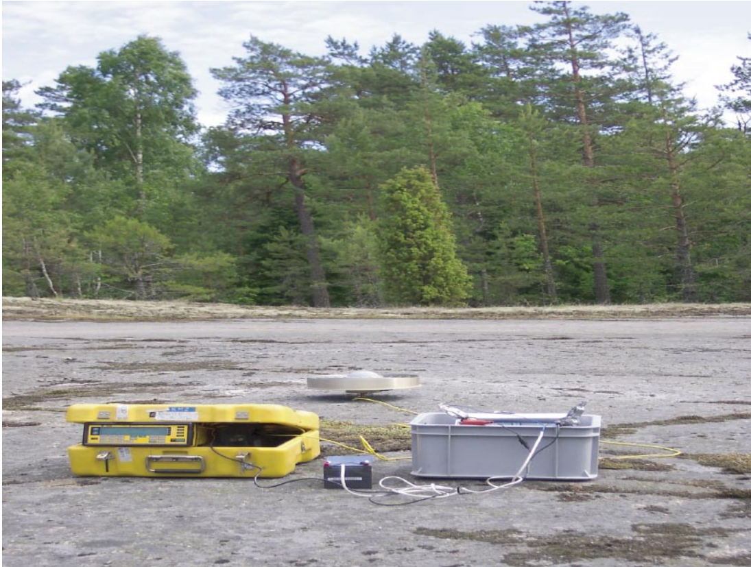
Figure 3-4. A choke ring antenna with a Trimble 4000 SSE GPS receiver at site Bast in June 2003.
