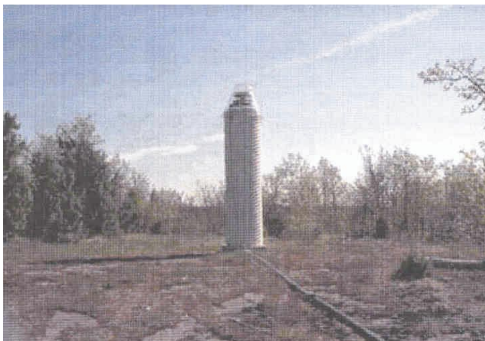
Figure 5-6. The SWEPOS station Oskarshamn with a choke ring antenna (with courtesy from SWEPOS).
