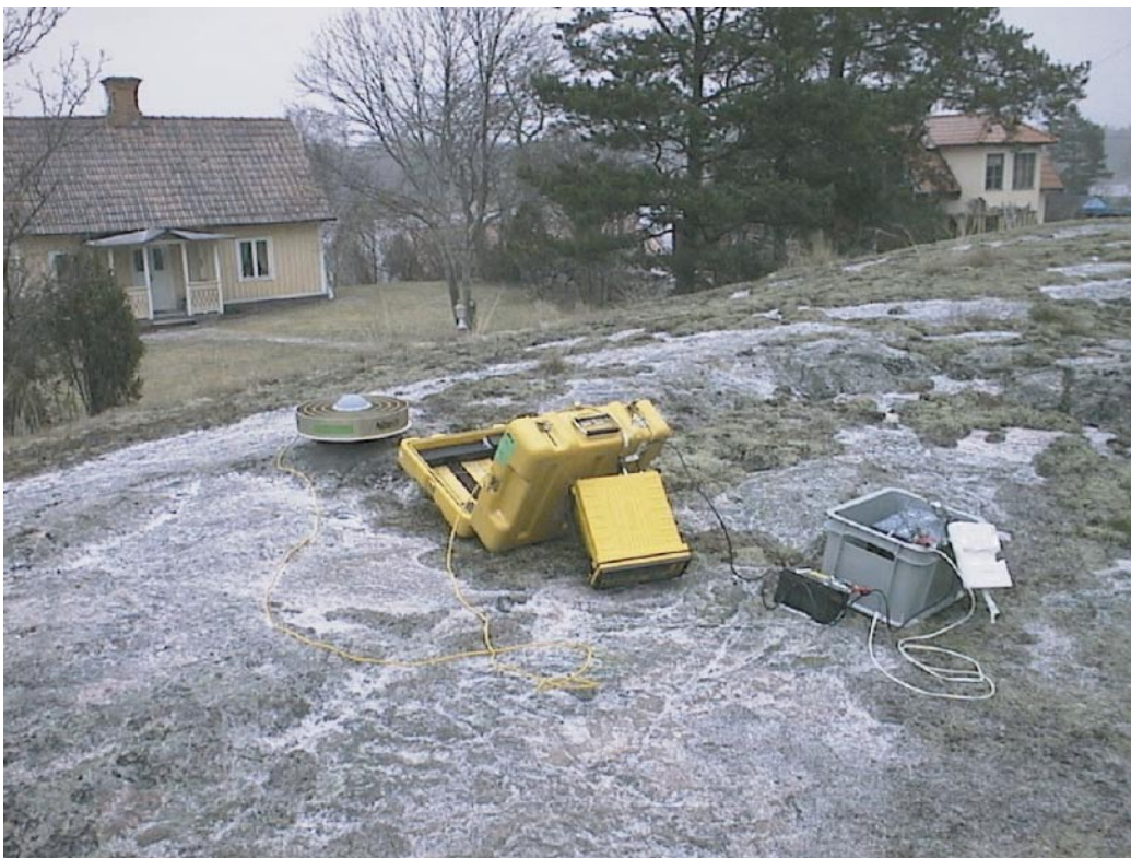
Figure 5-2. The receiver at site Karr slipped down from the box to the rock in June 2003. Fortunately, the cables were still connected and data was not lost.
