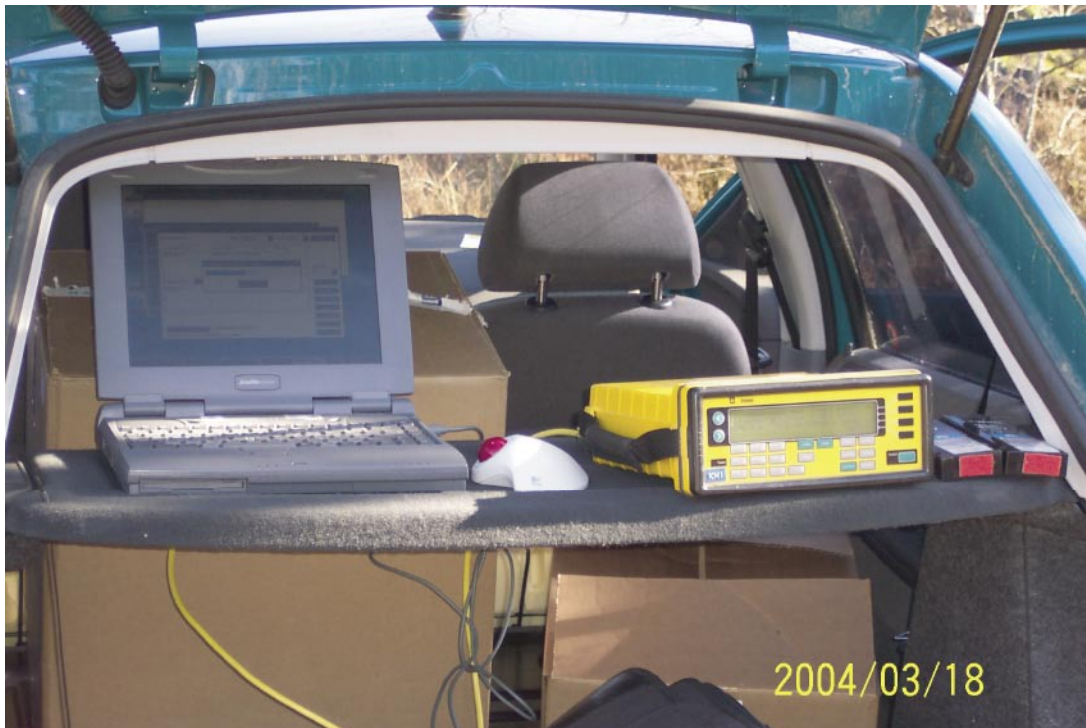
Figure 5-1. A personal field computer was transferring GPS data from a Trimble 4000 SSE receiver.
