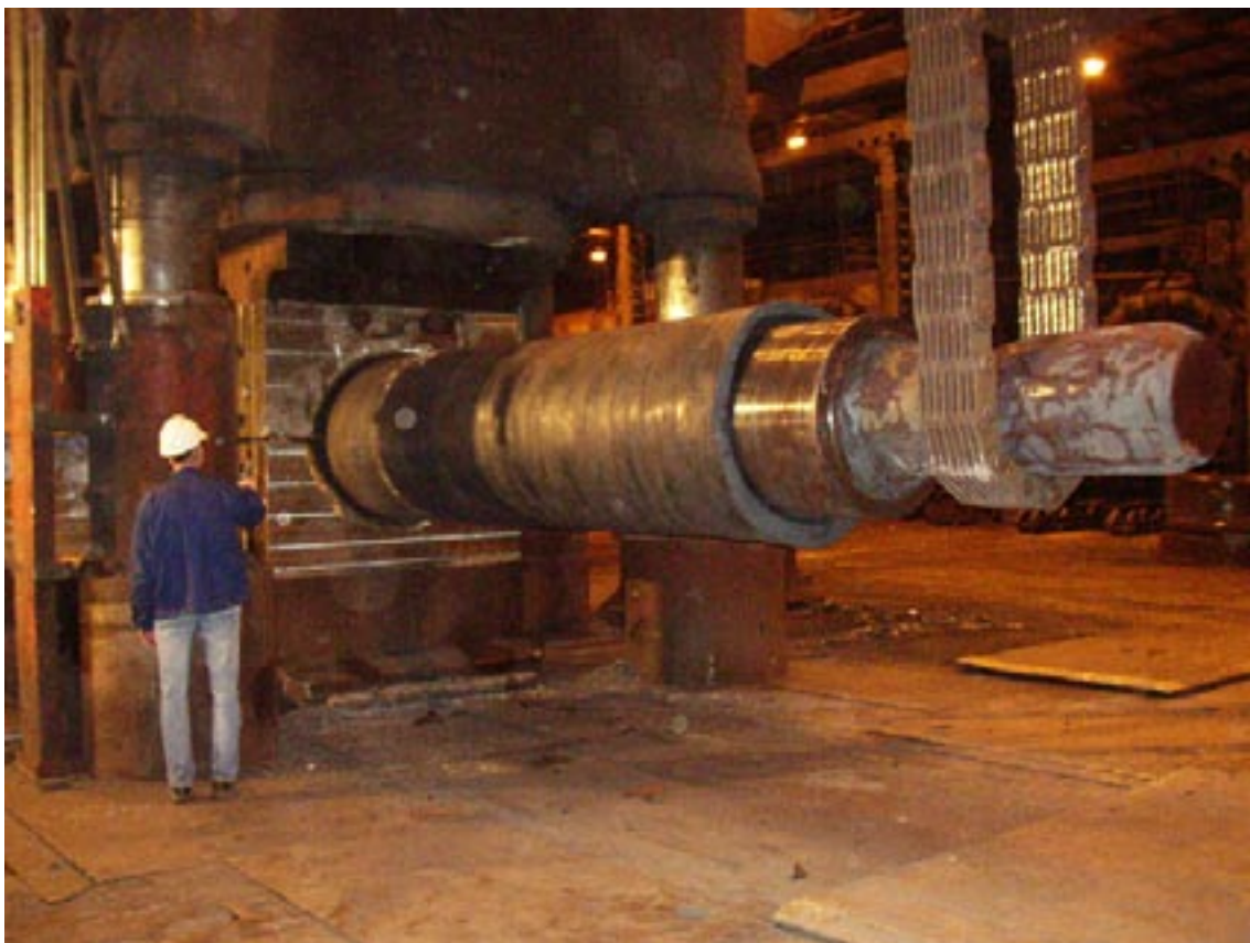
Figure 4-9. Final cogging operation in the concave die.
