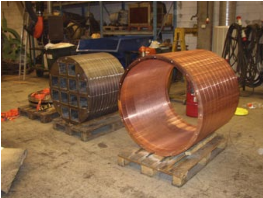
Figure 3-15. Part of insert I 26 and part of a copper tube for compression testing.
