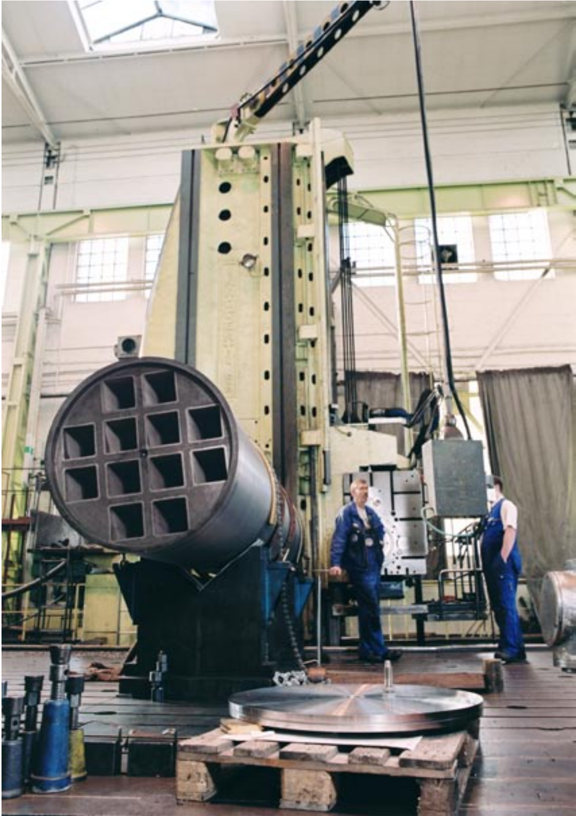
Figure 2-2. Steel lid for insert and a cast insert. The steel lid is designed to be screwed onto the insert with a bolt in the centre. The lid also has a groove for an O-ring to seal against the inside of the insert.
