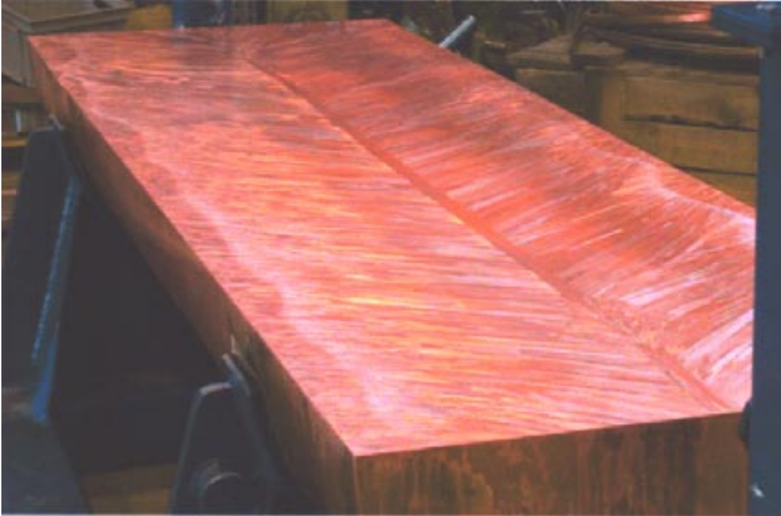
Figure 4-1. Crystal structure in a divided copper ingot.
