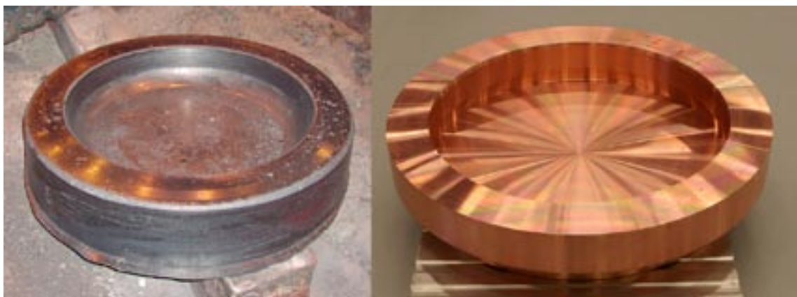
Figure 4-13 A and B. Photos of a finish-forged lid blank (A) and a lid no. TX 76, after machining (B).
