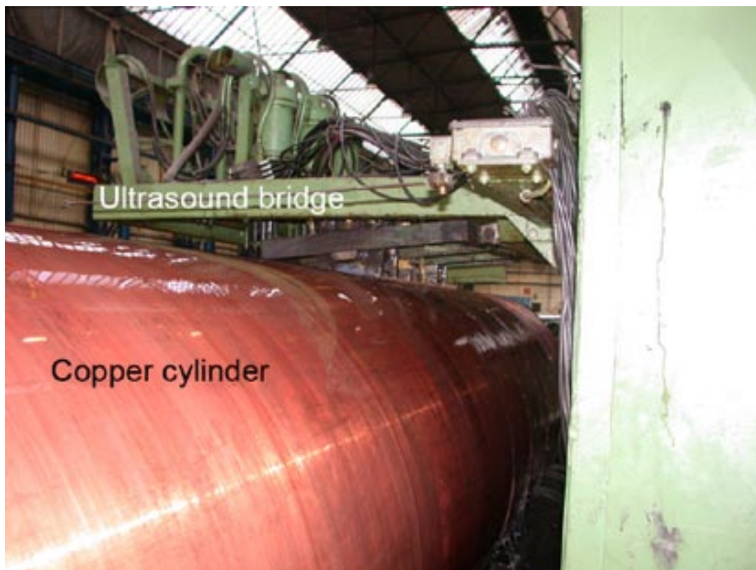
Figure 6-6. Test setup at Vallourec & Mannesmann Tubes.
