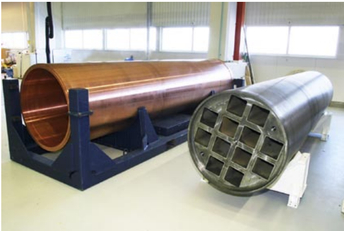
Figure 1-2. Copper tubes with welded bottom and cast insert.
