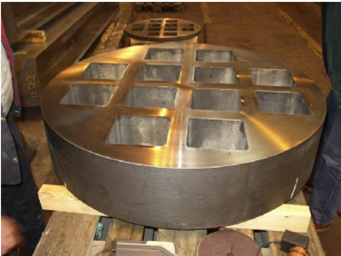
Figure 3-1. Discs cut from cast insert for material testing.
