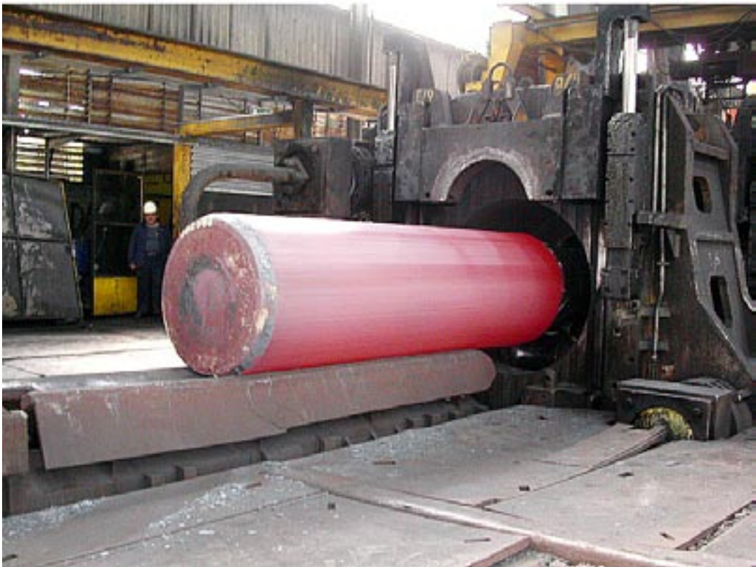
Figure 4-2. In pierce and draw processing, the copper tube is formed by a series of expansion steps and drawings to the desired size. The top picture shows an expansion and the bottom a drawing that elongates the tube.
