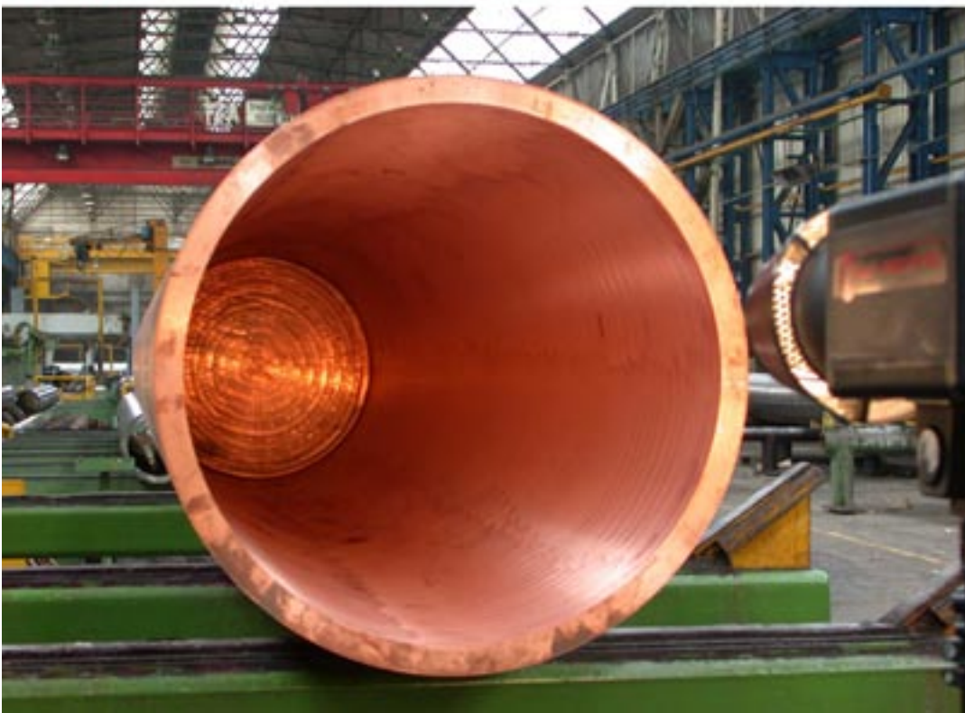
Figure 4-3 A and B. Tube T 34 with integral bottom after internal and external machining. See also reference /13/.
