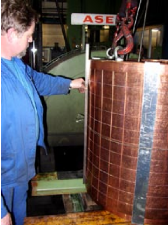
Figure 3-16. The test canister after being exposed to an isostatic pressure of 135 MPa. The copper shell has been deformed locally about 20 mm. But the canister is still intact.
