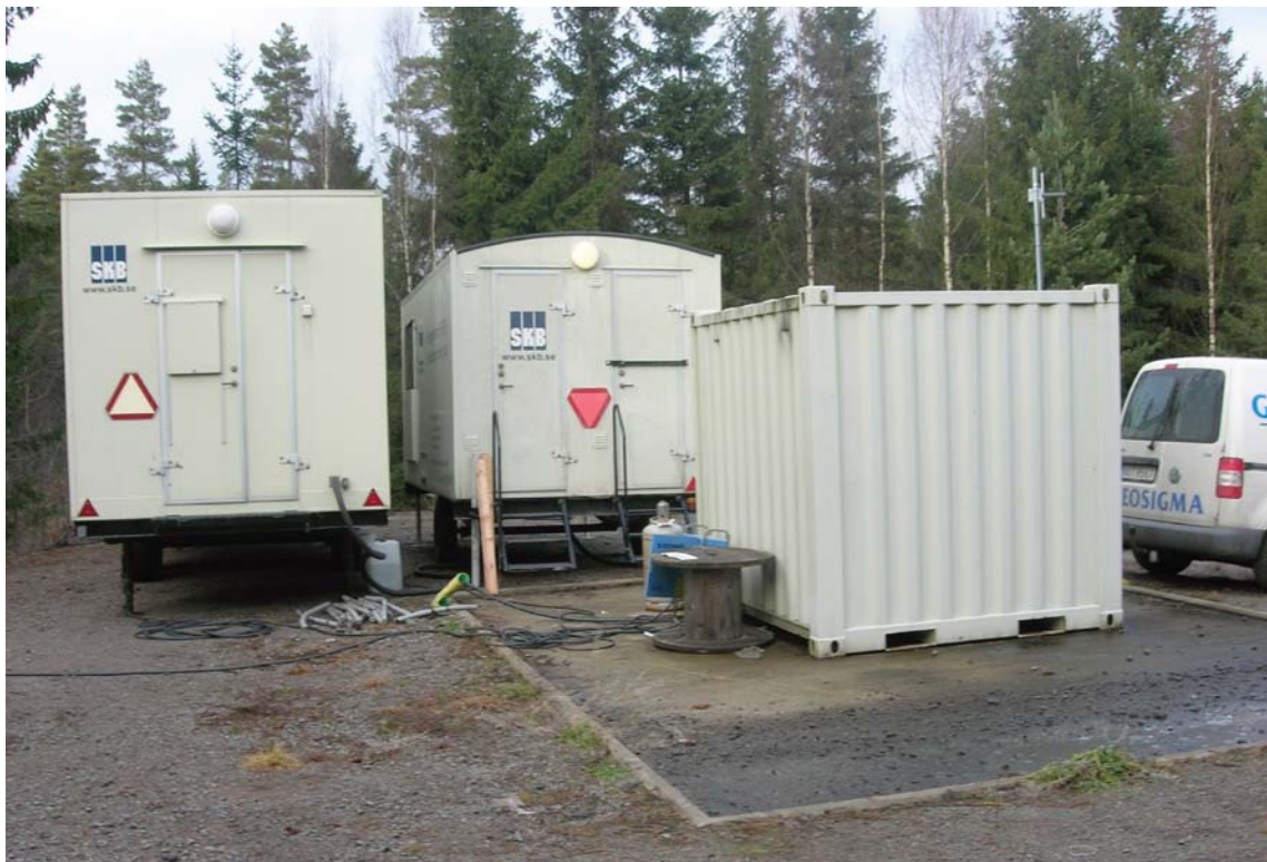
Figure 4-1. The mobile units used at KLX06; from left laboratory unit, unit for computer work and surface Chemmac with pH and redox electrodes. To the right the container with the installed borehole.
