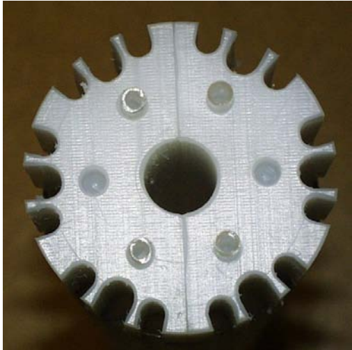
Figure 3-4. Cross section of a dummy (Ø76 mm). The tubing is placed in the tracks.
