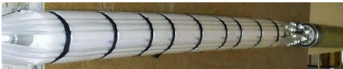
Figure 3-3. Dummy with attached tubing. Black tape (PVC) is used to keep the tubing together.
