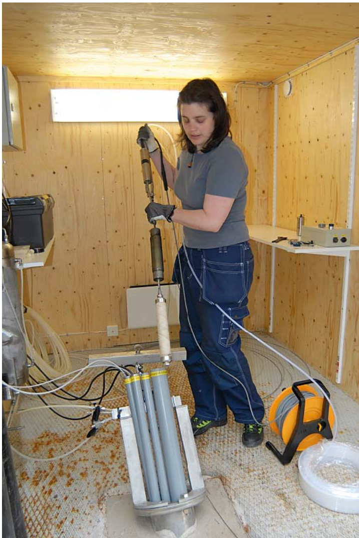
Figure 3-7. Lowering of sampling equipment in the standpipe in order to collect water from the connected borehole section. From bottom: filter, small inflatable packer and circulation pump. The standpipe with wider diameter is used for water sampling, while the standpipes with narrow diameter are used for pressure measurements.
