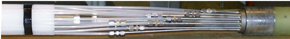
Figure 3-5. Detail between packer and dummy. The black tape that surrounds the couplings and tubing is missing in the picture.
