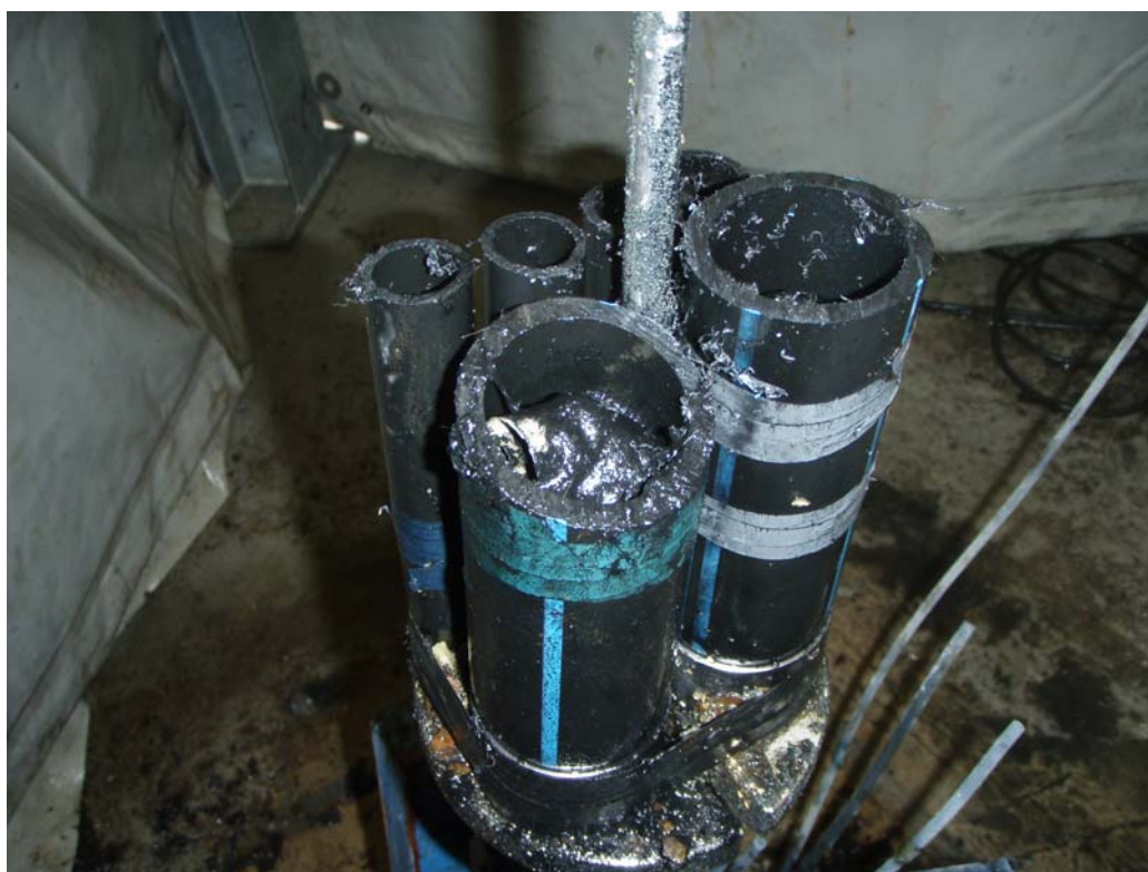
Figure A5-2. Standpipes in KAS03 with black precipitate. A strong smell of hydrogen sulphide gas.
