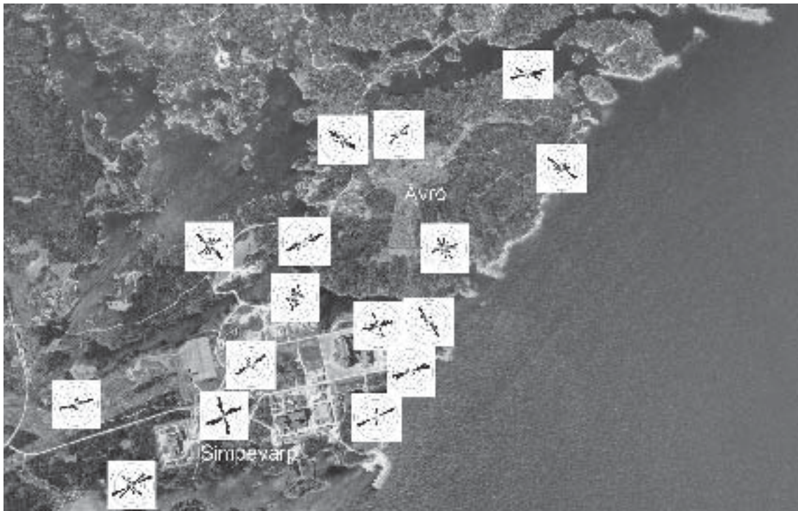
Figure 4-27. Orthophoto with diagrams showing fracture strike and frequency for fractures dipping 45 degrees or more at each outcrop.
