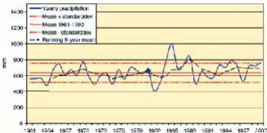
Figure 4-33. Annual precipitation, 5-year running average precipitation and mean of the total annual precipitation for the standard normal period 1961–1990, station Oskarshamn. Dashed lines: one standard deviation from the mean. /Larsson-McCann et al, 2002/.
