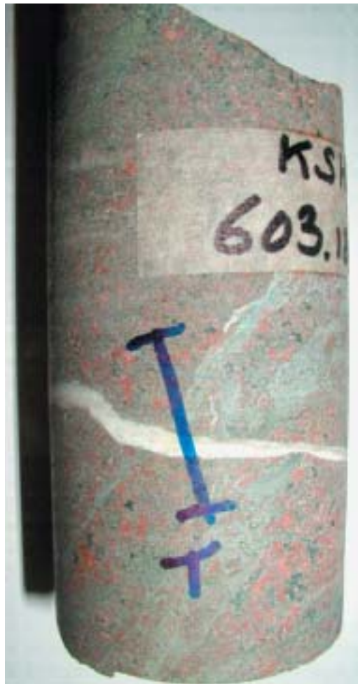
Figure 4-56. Drillcore sample KSH01A:603.11 m showing fracture sealed by prehnite (greenish) and cut by discordant calcite filling (white). Note the red staining and chloritisation of the wall rock. Blue line shows location of thin section.
