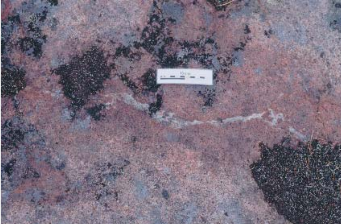
Figure 4-28. Red-staining along a sealed fracture in fine-grained dioritoid. The mineral infilling is thought to be dominated by prehnite.
