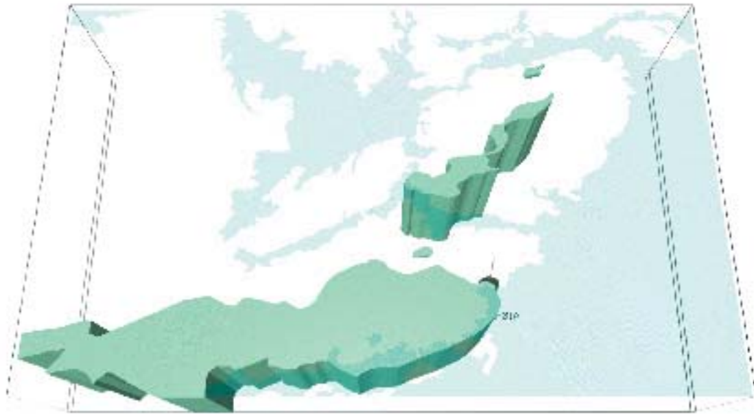
Figure 7-9. Alternative modelling of rock domains RSMB01 and RSMB03. Note the vertical contacts of the two major rock domains. View from the south.
