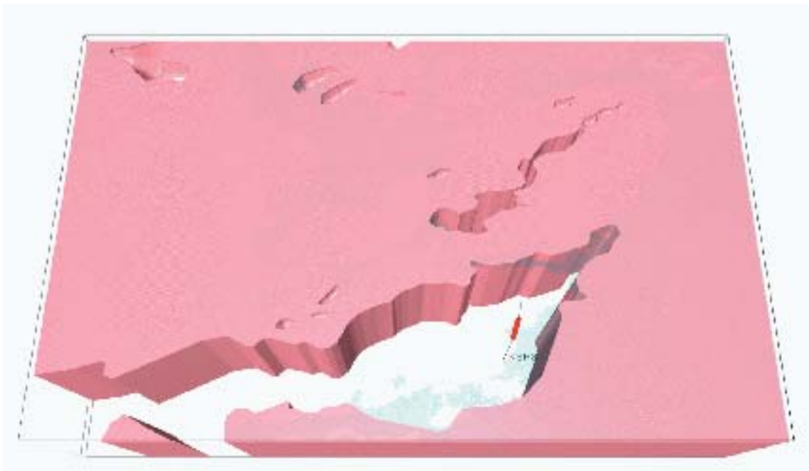
Figure 7-8. Alternative modelling of rock domain RSMA01. Note the vertical contacts between this rock domain and the other major rock domains. View from the south.
