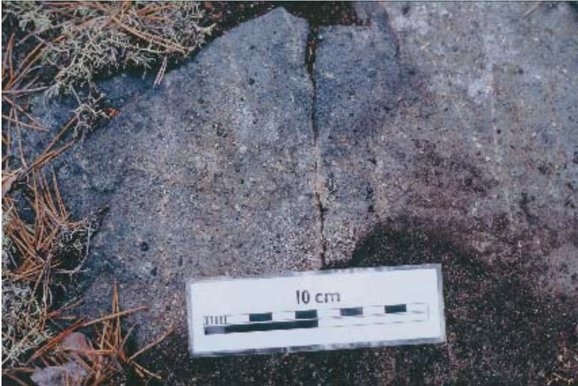
Figure 4-10. Fine-grained dioritoid with megacrysts of hornblende (dark grains) and plagioclase (white to light grey grains).
