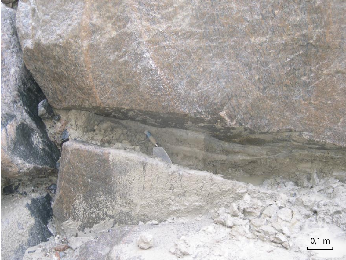
Figure 3-2. Sediment in bedrock fractures, as well as the till, was sampled by /Lokrantz and Albrecht/ in progress.
