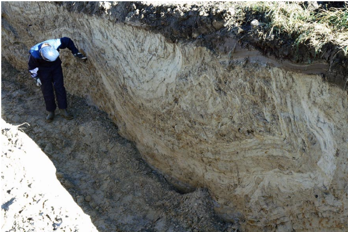
Figure 5-8. Abruptly cut folds in glacial silt at Marka (E6) indicate substantial erosion of a formerly thicker sequence.
