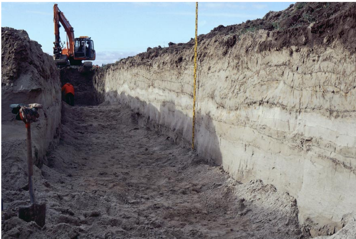
Figure 5-2. Typical for the stratigraphy along the Börstil esker, this trench section at Östansjö (E8) shows a bed of fine sand and coarse silt covered by a bed of clay-laminated silt. The uppermost 0.4 m consists of cultivated top-soil. Extended excavation revealed loosely packed and saturated glaciofluvial sand to a depth of at least 5 m. Although the stratigraphy is considered to be highly susceptible to liquefaction, no deformations related to seismically induced liquefaction were found here or elsewhere along the Börstil esker.
