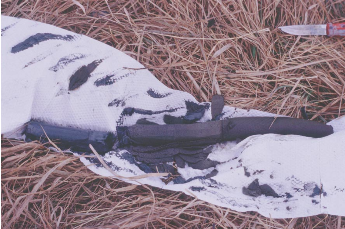
Figure 5-10. Sediment core from Söderängen (C3) consisting of an upper gyttja clay (right) and a lower bluish clay intercalated by a sandy layer. Graded bedding of sand and an unconformity between sand and underlying clay indicates erosion and deposition by a current of decreasing velocity.
