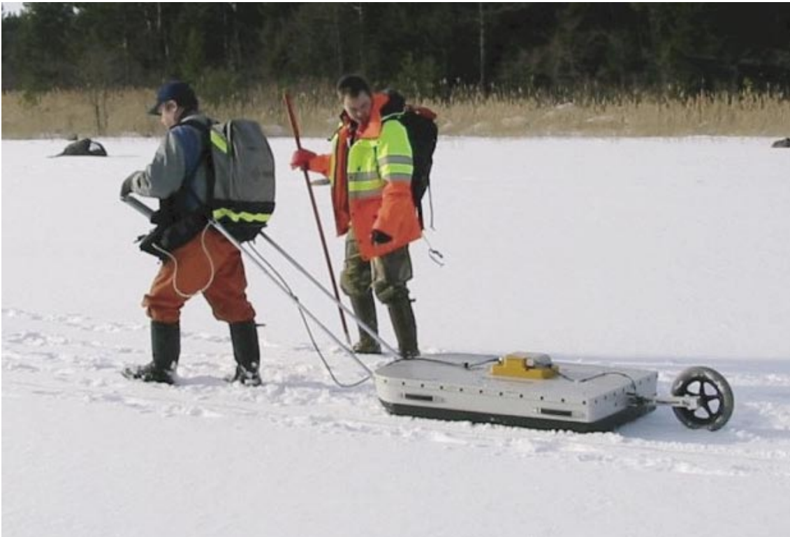
Figure 2-1. The GPR equipped with a 100 MHz antenna.
